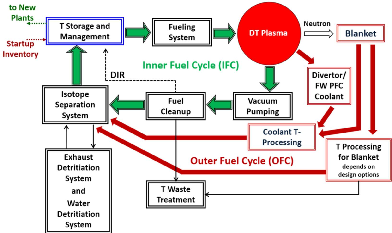
Simplified Schematic of the D-T Fuel Cycle
