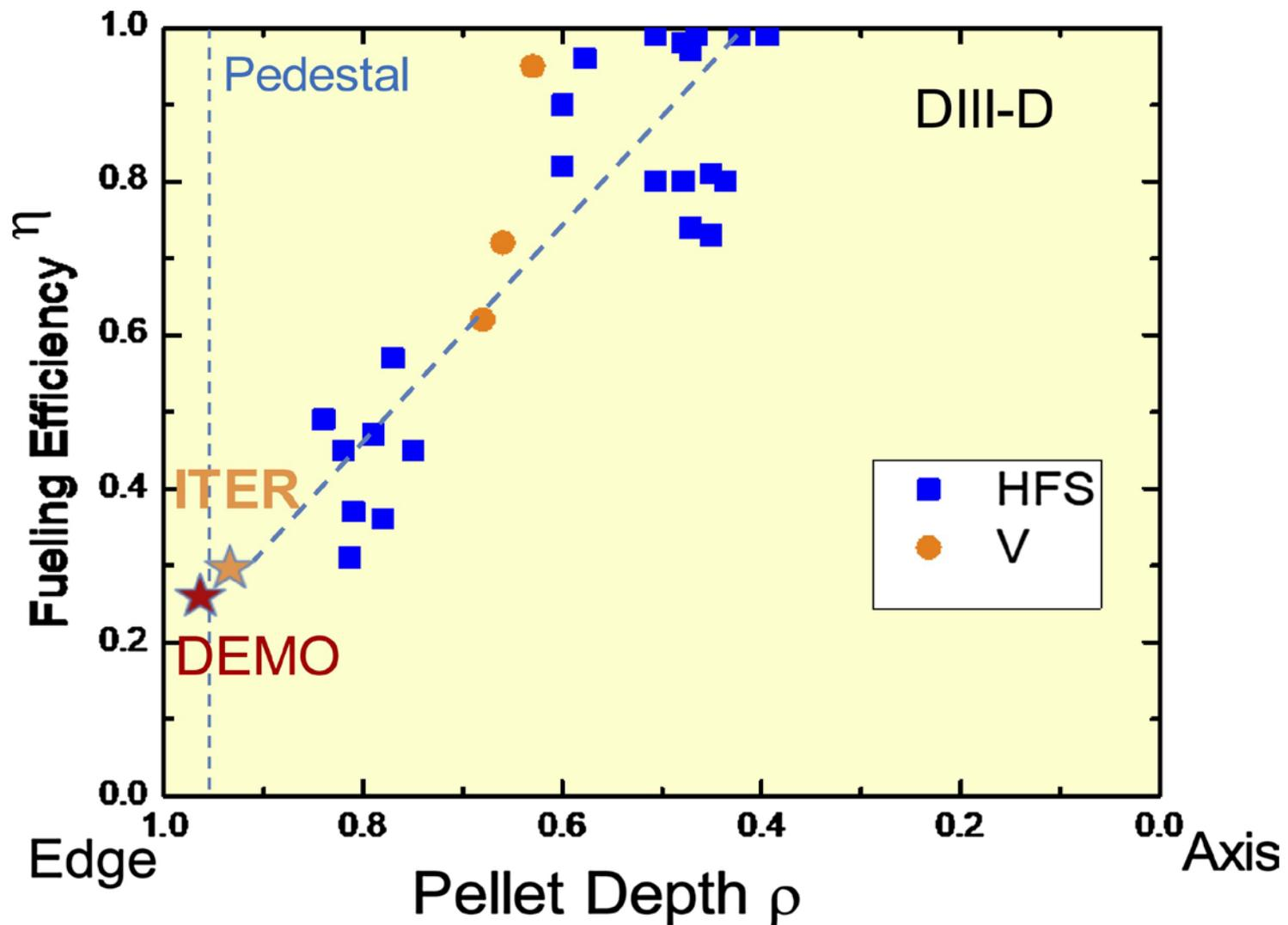
Fueling Efficiency **Extrapolation** from Deep to Shallow Penetrating Pellets Expected in ITER and DEMO is **Highly Uncertain**. Extrapolation shows fueling efficiency  $\eta < 25\%$  in ITER and even lower in DEMO Serious Consequences for required T start up and self-sufficiency
