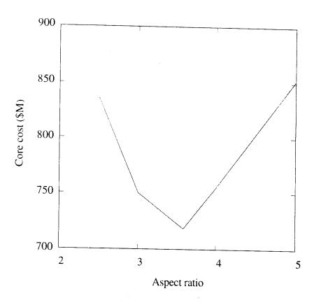
Fig. 1. VNS tokamak core cost versus aspect ratio.
