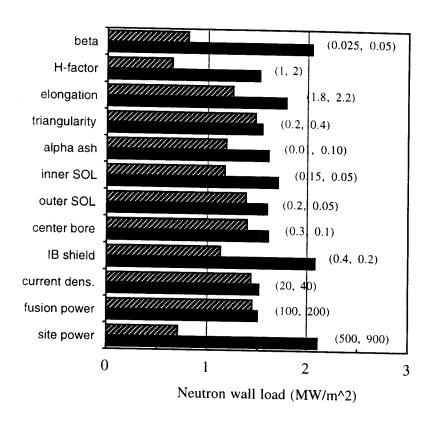
Fig. 3. Maximum average neutron wall load at bounding limits of design parameters.
