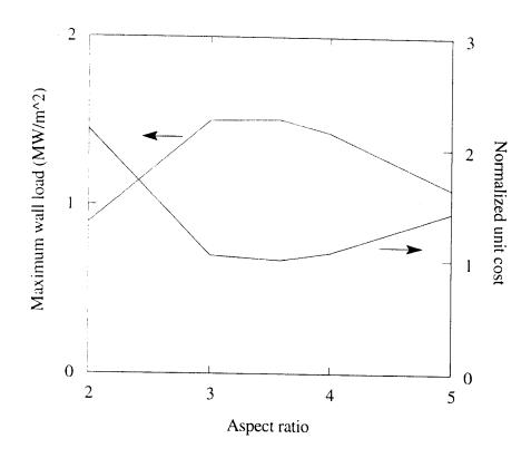
Fig. 2. Variations of maximum neutron wall load and normalized unit cost with aspect ratio.
