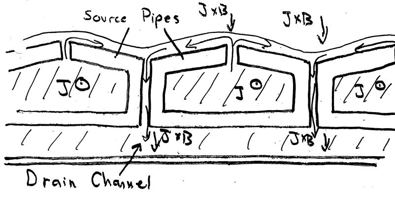
The source pipes are pressurized to force the liquid against MHD flow damping
