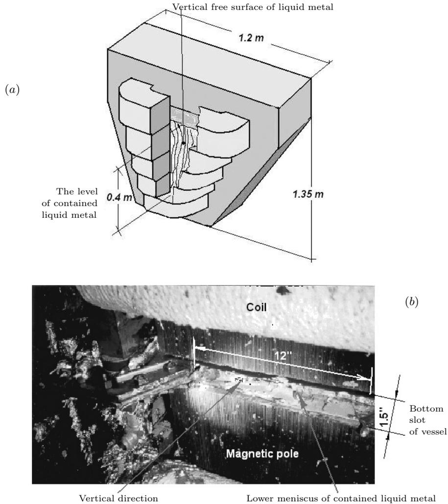
Fig. 4. MHD partial-levitation systems developed by Net Shape Cast, Inc.: (a) vertical free surface for the Twin Roll Strip Steel Caster for Inland Steel Inc. (USA), 1997, and (b) upside down Zn free surface for hot dip Zn-Al coating of steel strips and wires for Inland Steel, Inc. (USA), 2003, and for Danieli SpA (Italy), 2009.
