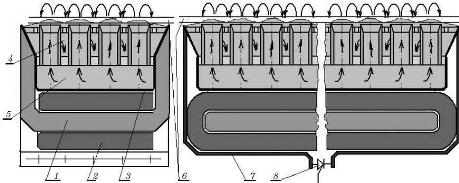
Fig. 6. Electromagnetic system of the “in-and-out honeycomb”: 1 - ferromagnetic core, 2 - AC fed coil, 3 - SS vessel with nozzles, 4 - drain duct, 5 - feeding duct, 6 - “forbidden zone” for preventing liquid metal splashes, 7 - copper current bypass, 8 - diodes.
