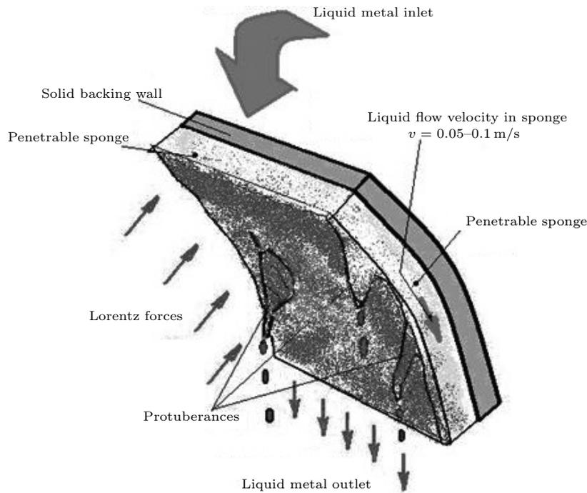
Fig. 3. Free-surface flow confinement in a porous structure (sponge) still evidences of liquid splashing if a magnetic field is applied.
