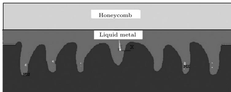
*Fig. 8.* The view of the upside down liquid metal surface in 0.2 s after energizing the inductor. The magnetic field below the free surface has not enough vertical gradient, hence, the electromagnetic field is not sufficiently large to prevent from leaking.
