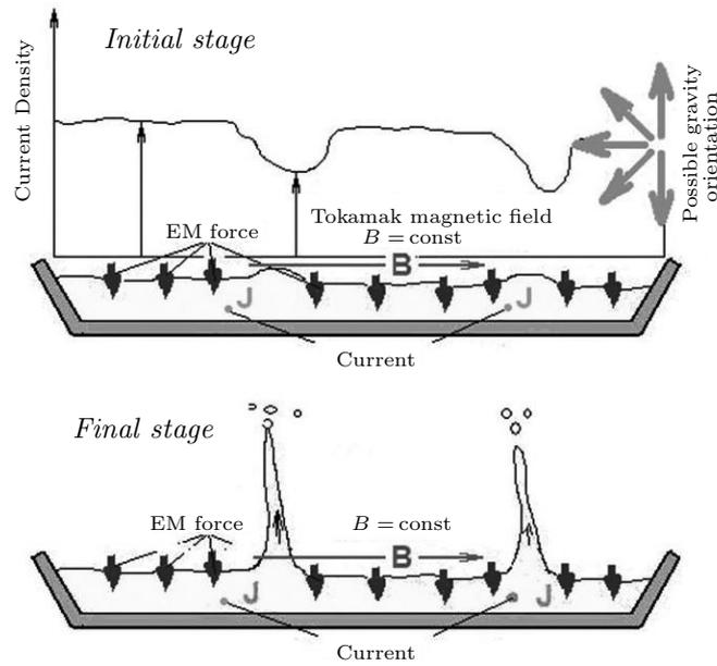
Fig. 2. Instability mechanism in the LM layer subject to a steady magnetic field and cross electric currents.
