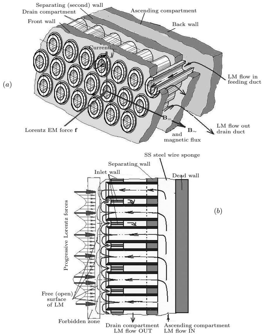
Fig. 5. The “in-and-out honeycomb” produces a free-surface film MHD flow to remove heat flux at the first wall or/and divertor: (a) conceptual design, (b) schematics of application of the retaining Lorentz force to the liquid metal in the vicinity of the free surface.
