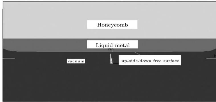
Fig. 9. Stable profile of the upside down liquid metal layer in a magnetic field with a vertical field gradient of 50 T/m.
