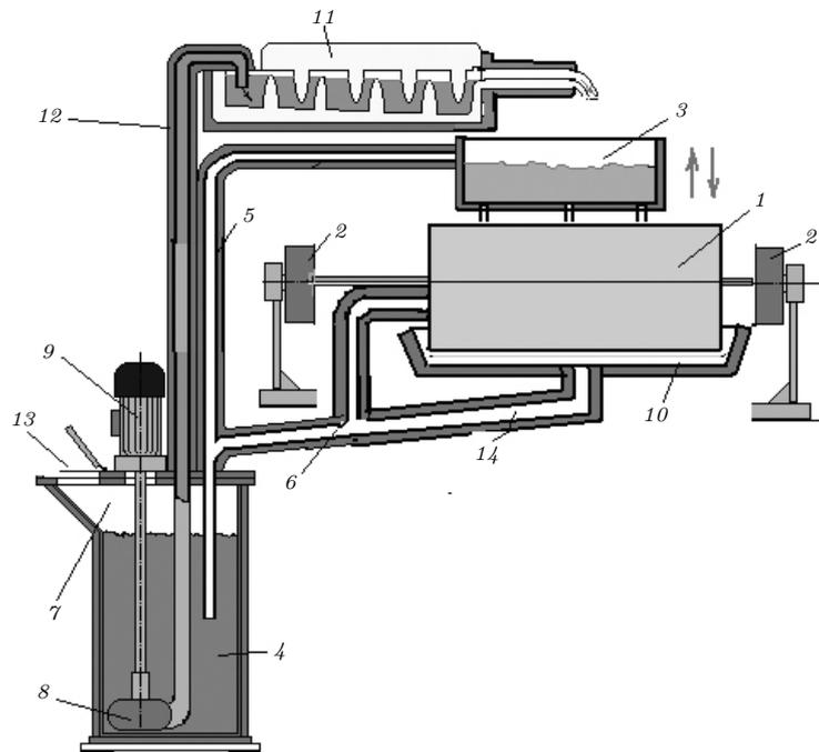
Fig. 7. The Sn-Bi circulation loop for in-and-out honeycomb module tests. 1 - in-and-out honeycomb, 2 - module tilting system, 3 - LM level control, 4 - melting oven/supply tank, 5 - overflow from LM level control, 6 - discharge pipe, 7 - space filled with nitrogen, 8 - liquid metal pump, 9 - pump motor, 10 - LM collector, 11 - sedimentation chamber, 12 - pressure feeder, 13 - hatch for loading chips, 14 - discharge pipe.
