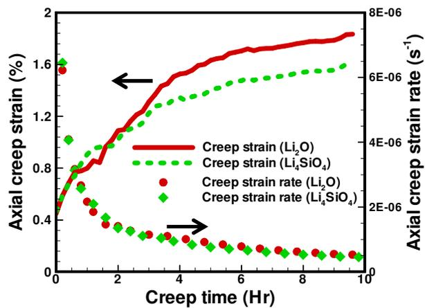
Figure 5 Axial creep strain and strain rate of  $\text{Li}_4\text{SiO}_4$  and  $\text{Li}_2\text{O}$  pebble beds under uniaxial pressure ( $P = 10\text{MPa}$ ).
