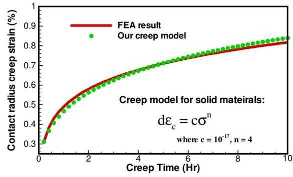
Figure 2 Verification of DEM creep model compared with FEA simulation of two particles.
