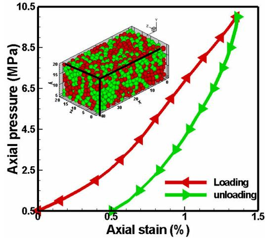
Figure 3 Stress-strain behavior of a rectangular pebble bed under uniaxial pressure (along y-direction).
