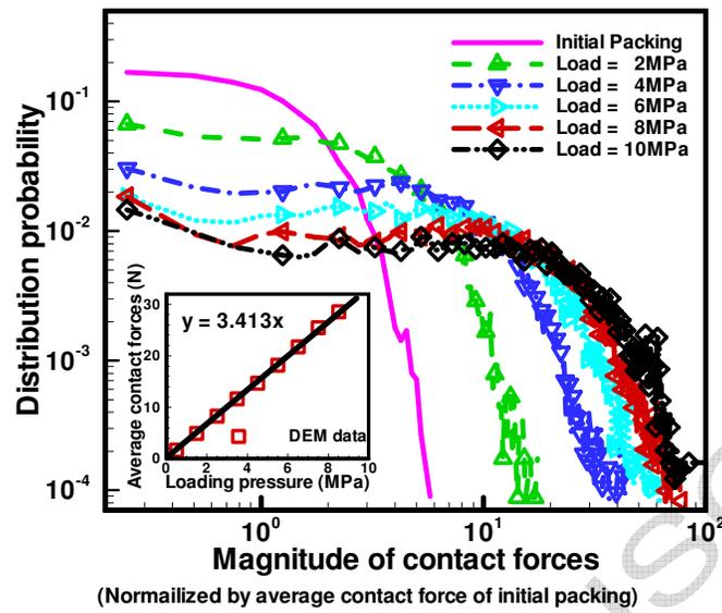
Figure 4 Distribution of particle contact force as a function of applied load. (The insert figure shows the magnitude relationship between average contact force and overall pressure.)
