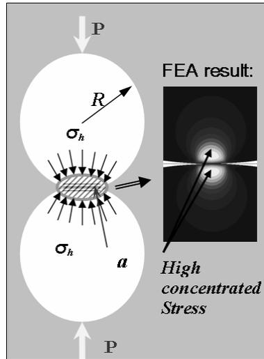
Figure 1 Sketch of two contacting particles. (The right insert figure shows a FEA simulation and light color areas stand for the highest stress.)
