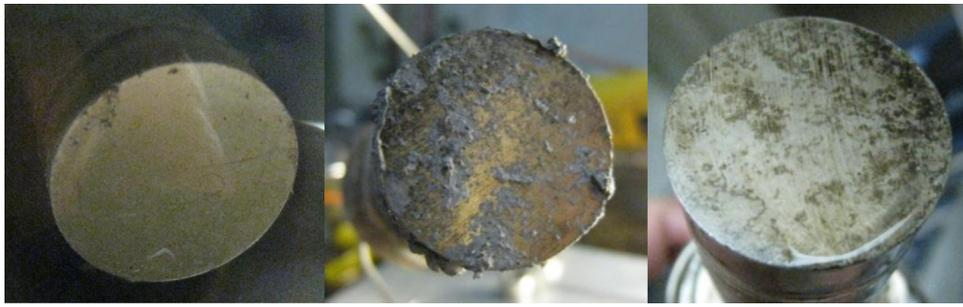
**Fig. 13.** Photographs of the titanium tip after submerging in PbLi at 450 °C: (left) after a few hours, (middle) after 290 h, (right) after removing PbLi residuals with a cleaning solution.
