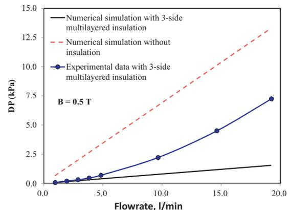
**Fig. 16.** Low magnetic field pressure drop: experiment versus computations.
