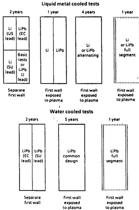
FIG. 2. Test sequence for liquid metal blankets.
