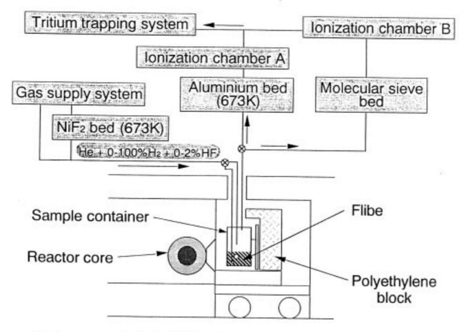
TF is converted to HT in the aluminium bed and the concentration of all released tritium (HT and TF) is monitored by the ionization chamber A.
