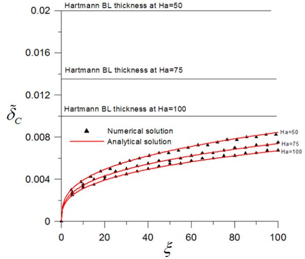
Fig. 2. Comparison for the thickness of the concentration boundary layer in the Zone I between analytical and numerical solutions at  $Pe_D = 10^8$ .
