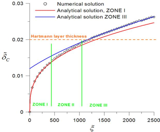
Fig. 3. Comparison between the numerical solution and the analytical solutions for Zones I and III for  $Ha=50$ ,  $Pe_D=10^8$ .
