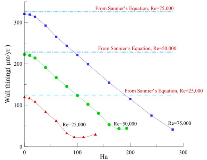
Fig. 1. Comparison of the computed wall thinning with the predictions from Sannier’s equation for the case of a wall-normal magnetic field at 500°C.
