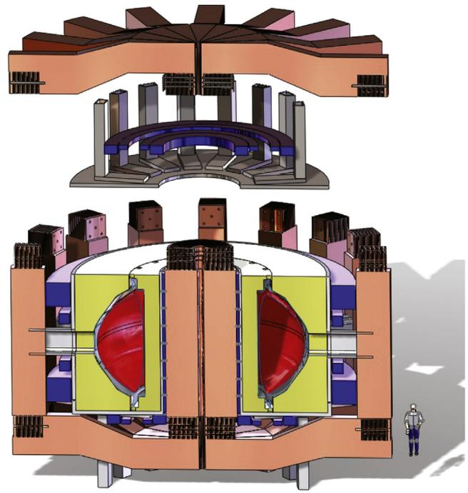
**Fig. 1.** Baseline maintenance scheme for FNSF-AT is based on vertical crane lift of toroidally continuous ring structures.
