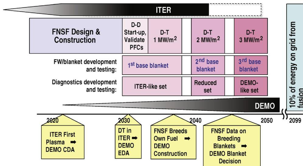
**Fig. 2.** A staged development to learning and improving nuclear components, diagnostics, and operating scenarios enables an early start for FNSF that maximizes synergy with the parallel ITER program: the “fast-track” approach.
