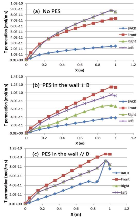
Fig. 11. Tritium permeation per unit length through the LM\_FS walls (the front, back, left and right walls).
