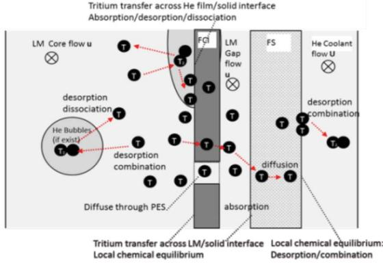
Fig. 1. The schematic of the tritium transport model shows all the sources and transportation modes of tritium in a liquid metal breeder blanket unit.
