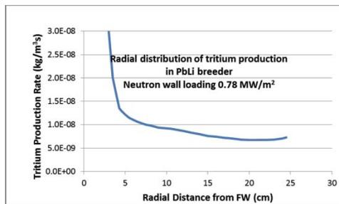
Fig. 6. Tritium generation rate shows a non-uniform profile along the radial distance from FW.
