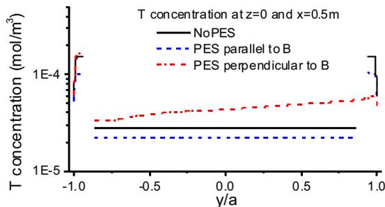
Fig. 10. Tritium concentrations along the line of  $z=0\text{m}$  at the cross-section of  $x=0.5\text{m}$  shows higher concentrations in the gaps than in the core.
