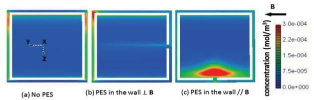
Fig. 7. Tritium concentrations at across section of  $x=0.5m$  for various PES configurations.
