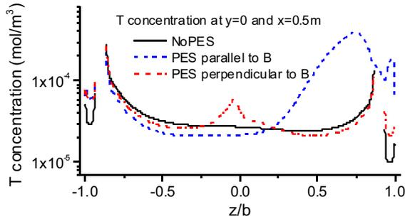
Fig. 9. Tritium concentrations along the line of  $y=0\text{m}$  at the cross-section of  $x=0.5\text{m}$  shows a high tritium concentration in the bulk area near the location of the PES for the case of PES is opened parallel to the field
