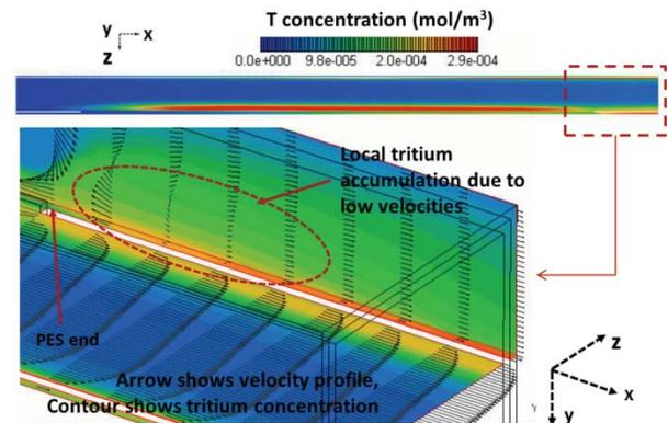
Fig. 8. Tritium concentration near the outlet (bottom) and at the cross-section of  $y=0$  (top) with PES wall parallel to the field. Here Tritium accumulated in the core area above the PES and in the back gap behind the PES end.
