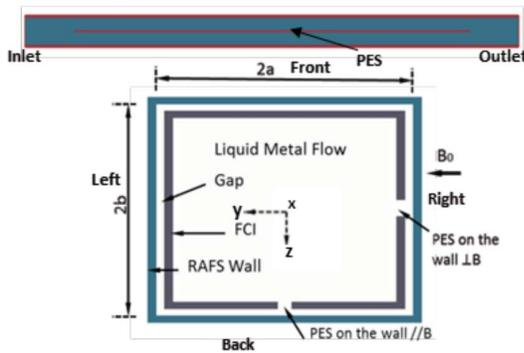
Fig. 2. The cross-section drawing of the blanket duct shows the PES openings. Here the PES is opened from  $x=0.1m$  to  $0.9m$  and with  $2a=0.06m$ ,  $2b=0.06m$ , RAFS wall  $0.002m$ , FCI  $0.002m$ , PES  $0.003m$ , Gap  $0.002m$
