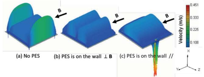
Fig. 4. Velocity profiles at across section of  $x=0.5m$  for various PES configurations.
