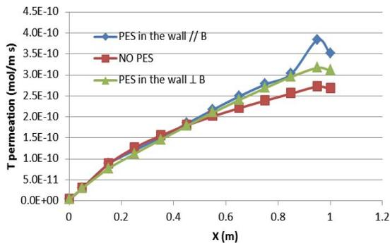
Fig. 12. Total tritium permeation per unit length through LM-FS walls
