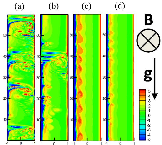
Fig. 2. Vorticity snapshots in a turbulent mixed-convection flow. Strong turbulence: (a)  $Ha = 50, Gr = 10^8, Re = 5000$ ; (b)  $Ha = 75, Gr = 10^8, Re = 7500$ . Weak turbulence: (c)  $Ha = 75, Gr = 5 \times 10^7, Re = 10,000$ ; (d)  $Ha = 120, Gr = 10^8, Re = 5000$ .
