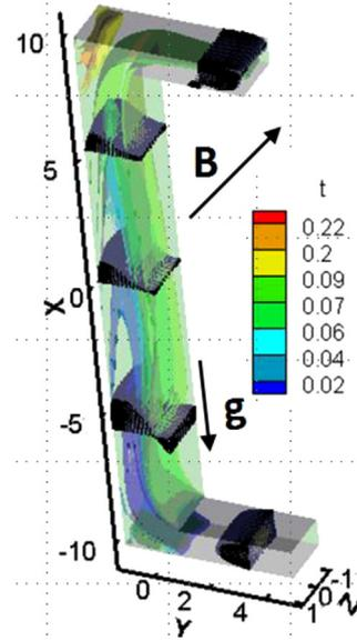
Fig. 1. 3D velocity vectors and temperature counters at  $Ha = 70, Gr = 10^8, Re = 10,000$ .
