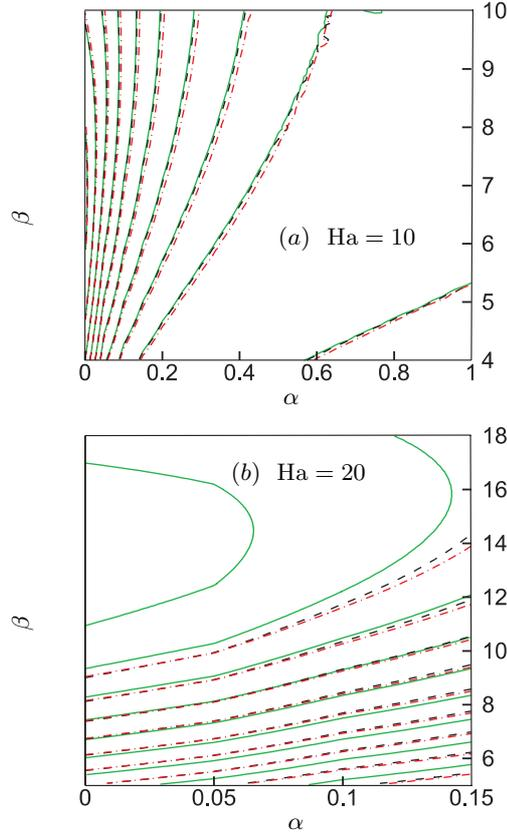
Fig. 4. Isovalues of  $G_{\max}(\alpha, \beta)$  for  $\text{Re} = 40\,000$  in three cases: no-slip (solid), symmetric slip with  $\lambda_1 = 0.001$  (dash) and with  $\lambda_1 = 0.003$  (dash dot). The values of  $G_{\max}$  are (a) 1000, 3000 to 11000, (b) 800 to 2400 in steps of 200 from outer to inner curve.
