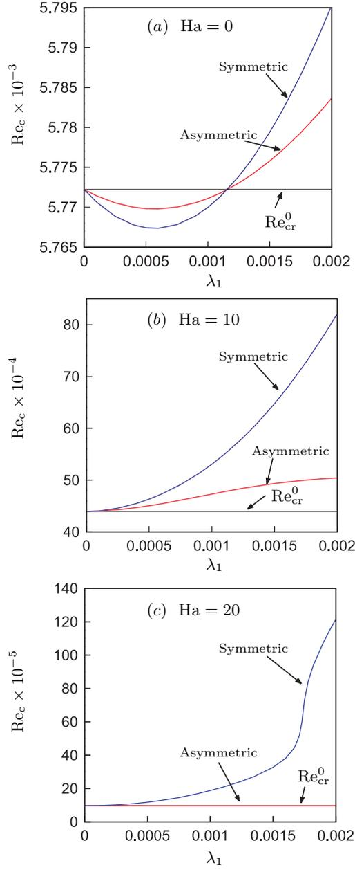
Fig. 2. Variation of the critical Reynolds number with the non-dimensional slip length for the symmetric and asymmetric slip cases.
