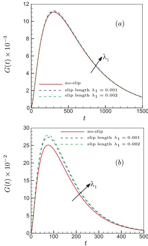
Fig. 5. Maximum energy growth rate at  $\text{Re} = 40\,000$  with different slip lengths in the symmetric slip case. (a)  $G(\alpha = 0, \beta = 6.8)$  for  $\text{Ha} = 10$ ; (a)  $G(\alpha = 0, \beta = 13.65)$  for  $\text{Ha} = 20$ .
