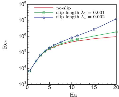
Fig. 3. Near exponential increase of the critical Reynolds number with the Hartmann number.
