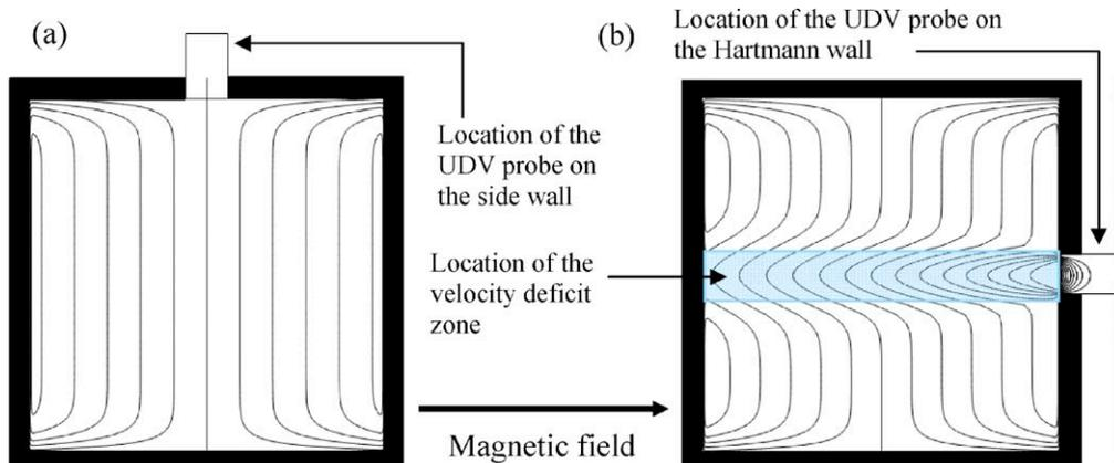
Fig. 8. Effect of the conducting HT-UDV probe on the induced electric current: (a) probe located on the side wall, and (b) on the Hartmann wall (b) of the host rectangular duct.
