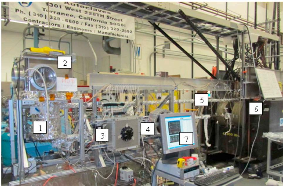
**Fig. 1.** Newly-constructed MHD PbLi loop at UCLA: 1 – PbLi melting tank with heaters, 2 – glove box, 3 – EM pump, 4 – EM flow-meter, 5 – pipes, 6 – electromagnet, and 7 – data acquisition system.
