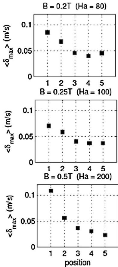
Fig. 7. Velocity fluctuations in the largest channel as a function of the axial position at  $Re = 54,000$  ( $0.4$  m/s).
