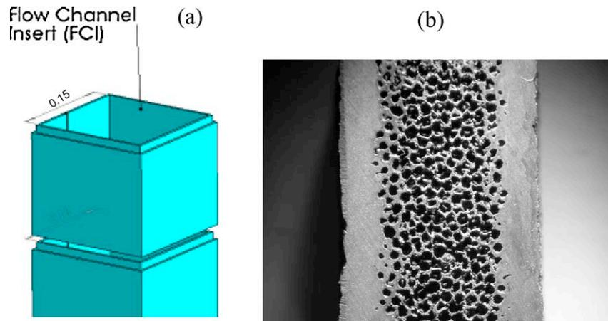
Fig. 5. SiC FCI: (a) schematic view of two overlapping FCI sections, and (b) foam-based SiC sample.
