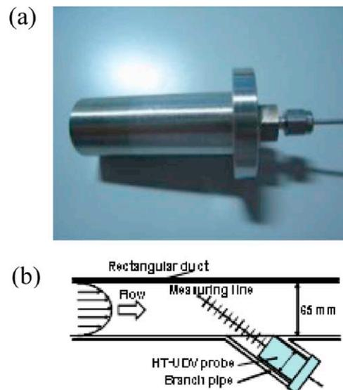
**Fig. 4.** (a) HT-UDV probe and (b) its location in the test-section.
