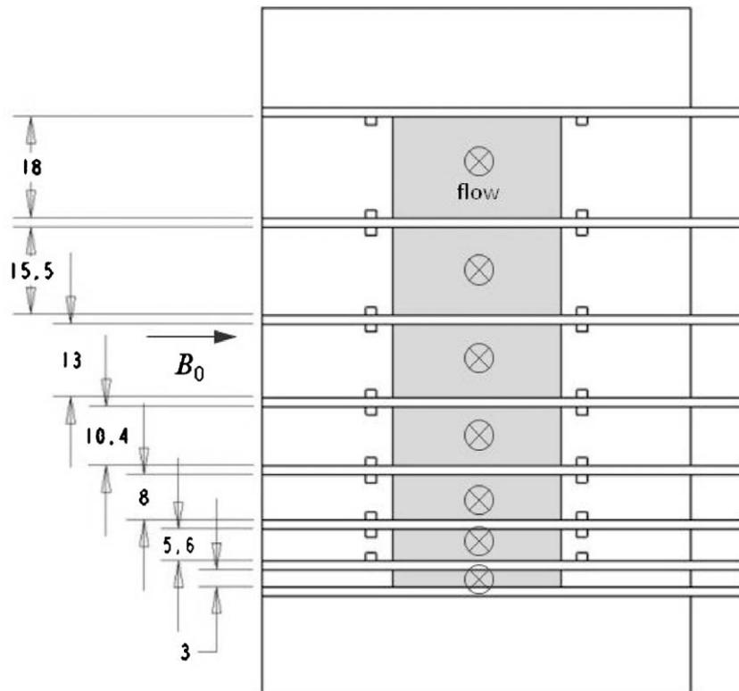
Fig. 6. Stack of 7 channels in the pre-qualification experiment.
