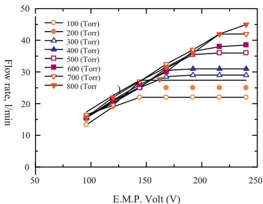
**Fig. 3.** Testing the EM pump. Flow rate is increased up to 50 l/min as the pump voltage is increased. Measurements are performed for the argon pressure from 100 to 800 Torr.
