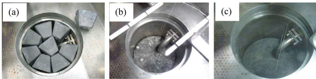
**Fig. 2.** Melting PbLi: (a) PbLi ingots before melting, (b) bubble formation during melting and further heating, and (c) oxide crust 0.5–1 cm thick with clean PbLi beneath.
