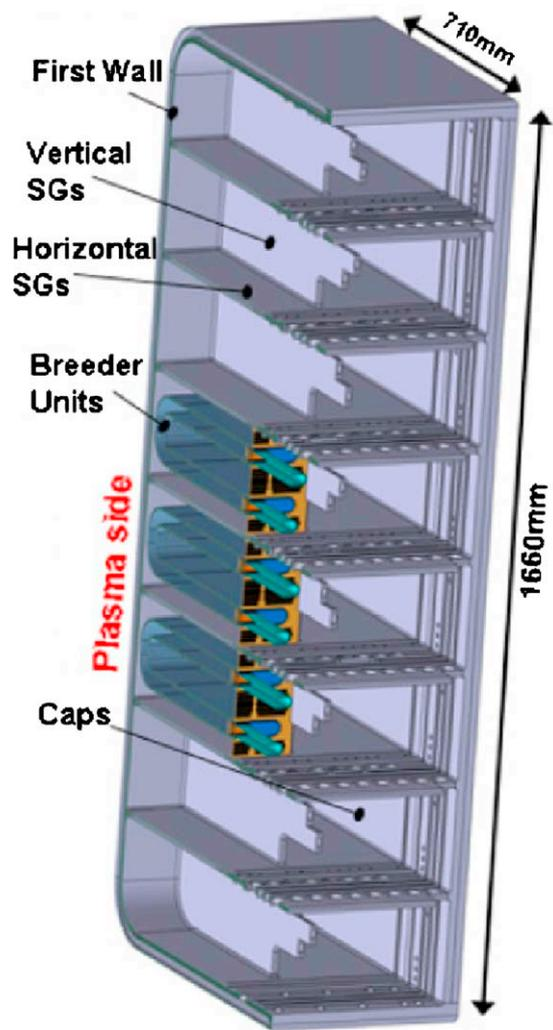
Fig. 2. Internal view of the HCPB-TBM.
