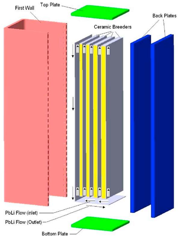
Fig. 6. Exploded view of the LLCB-TBM.
