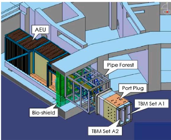
Fig. 7. View of the TBM port cell area.
