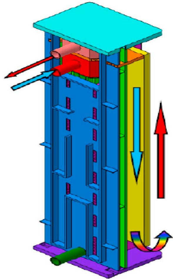
Fig. 4. Details of the Pb-16Li path in the DCLL-TBM.
