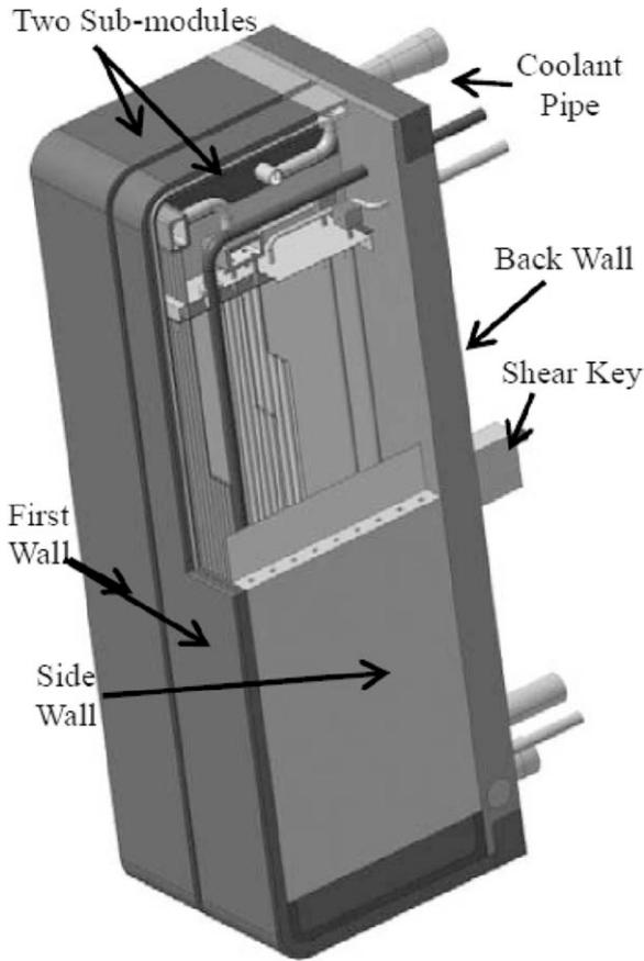
Fig. 3. View of the WCCB-TBM.
