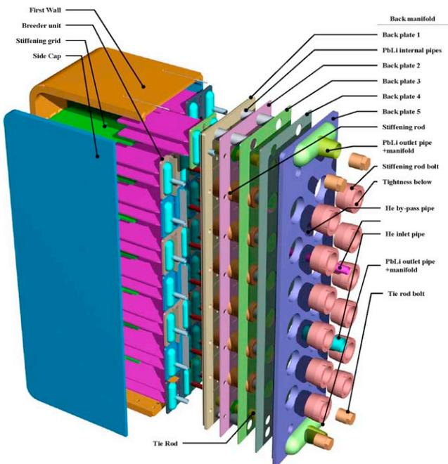
Fig. 1. Exploded view of the HCLL-TBM.
