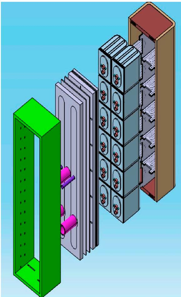
Fig. 5. Exploded view of the HCCB-TBM.
