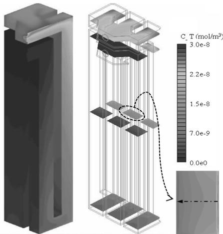
Fig. 7. Contour plots of the tritium concentrations ( $\text{mol/m}^3$ ) in simplified DCLL TBM channels with toroidal magnetic field and radial distributed tritium production.
