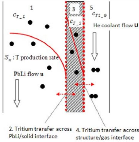
Fig. 1. Schematic of the tritium transport model.
