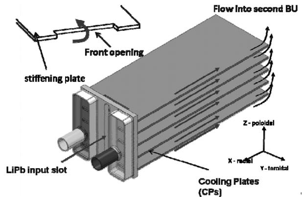
Fig. 9. HCLL breeder unit geometry.
