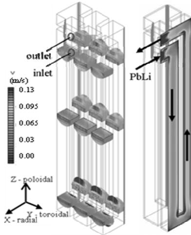
Fig. 6. Velocity profile in simplified DCLL TBM channels with toroidal magnetic field
