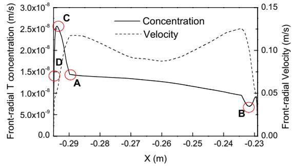
Fig. 8. The tritium concentration and the corresponding velocity profile are plotted as a function of the radial direction along the center line of the geometry at the front channel indicated by dotted arrow in Fig. 7
