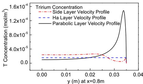
Fig. 4. Tritium concentrations along y-direction at x=0.8m for parabolic, side and Hartman layer velocity profiles.
