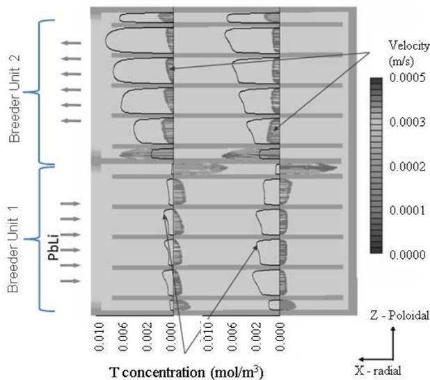
Fig. 10. The tritium concentration and the corresponding velocity profile at the middle plane of the geometry.
