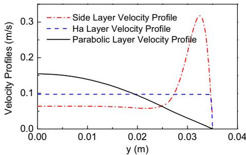
Fig. 3. Parabolic, side layer and Hartman layer velocity profiles along y-direction at same mass flow rates 22kg/s.
