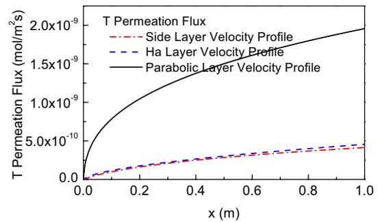
Fig. 5. Tritium permeation flux along wall for parabolic, side layer and Hartman layer velocity profiles.
