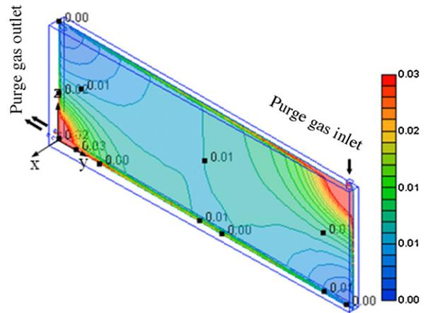
Fig. 5. The velocity field in the purge gas region at the  $x=0.012$  m plane.
