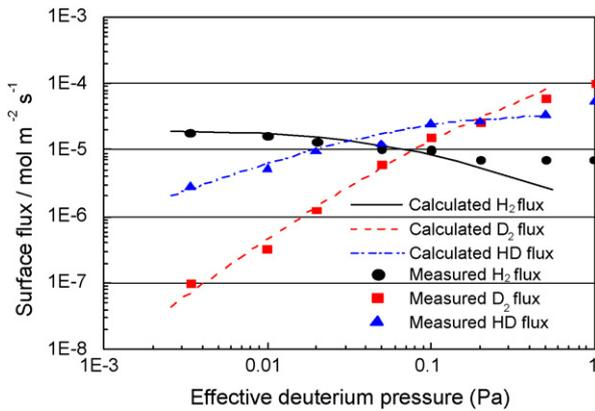
Fig. 3. HD, H<sub>2</sub>, D<sub>2</sub> permeation flux in co-permeation measurements as a function of the effective deuterium pressure ( $P_D = P_{D_2} + P_{HD}/2$ ) and at a fixed value of effective H<sub>2</sub> pressure ( $P_H = P_{H_2} + P_{HD}/2 = 0.063$  Pa).
