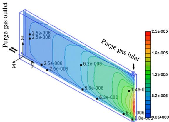
Fig. 7. Tritium concentration in the purge gas region at the x=0.012 m plane.
