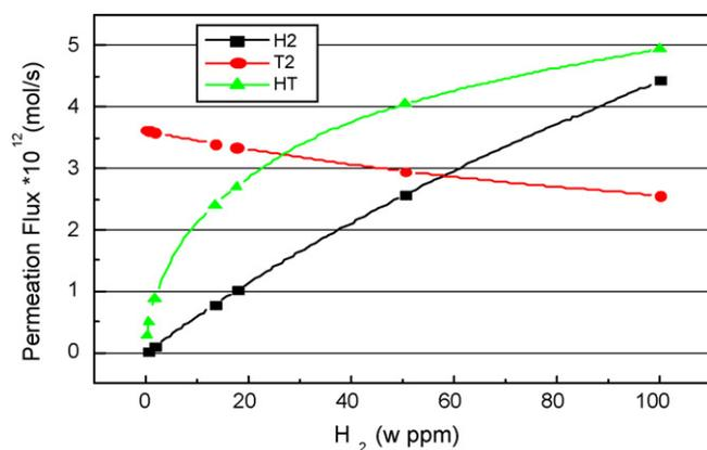
**Fig. 11.** Permeation flux of H<sub>2</sub>, T<sub>2</sub>, and HT molecules as a function of the amount of H<sub>2</sub> added.
