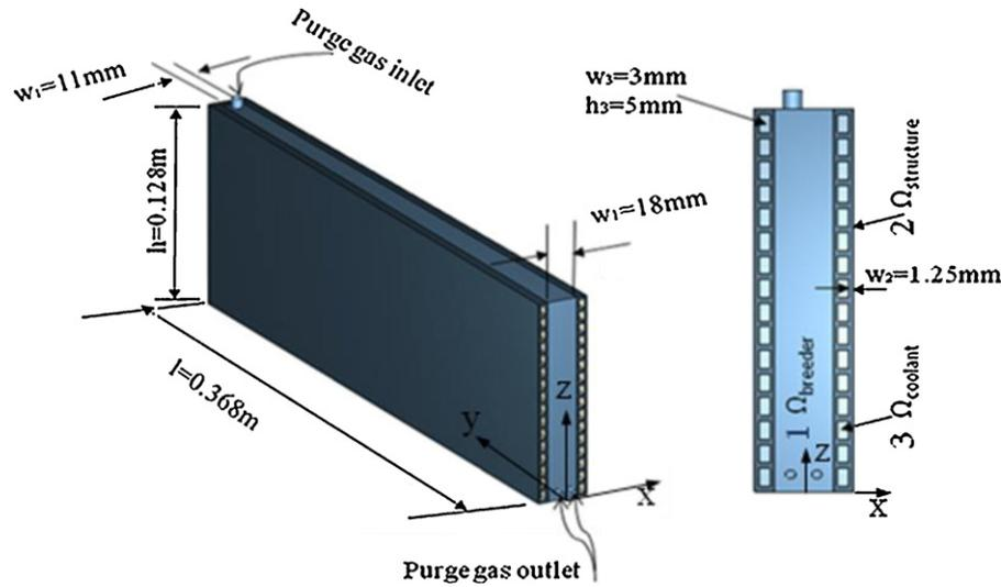
Fig. 1. Diagram of the blanket module.
