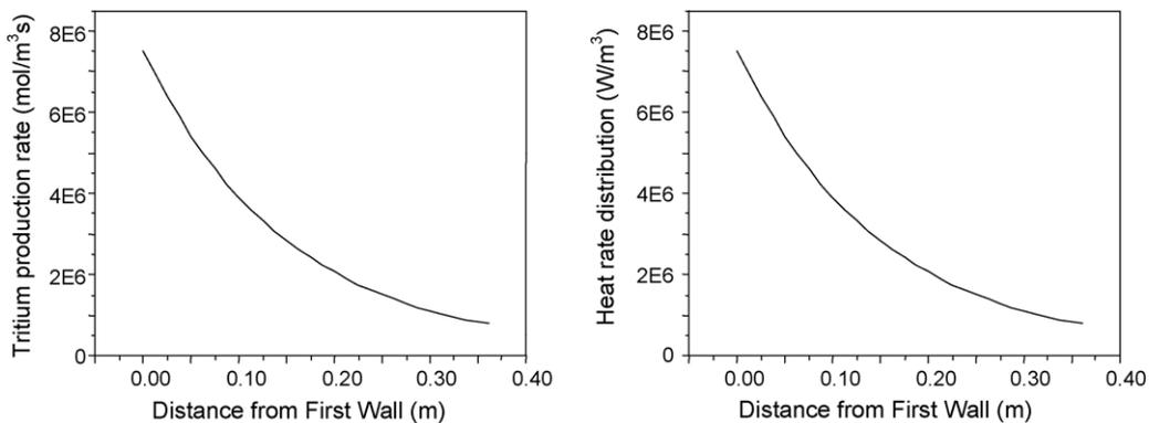
Fig. 4. Nuclear heating rate and tritium production rate as a function of distance in the radial direction.
