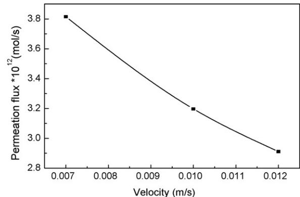
Fig. 10. The total tritium permeation flux through the purge gas–structure interface at different average flow velocities.
