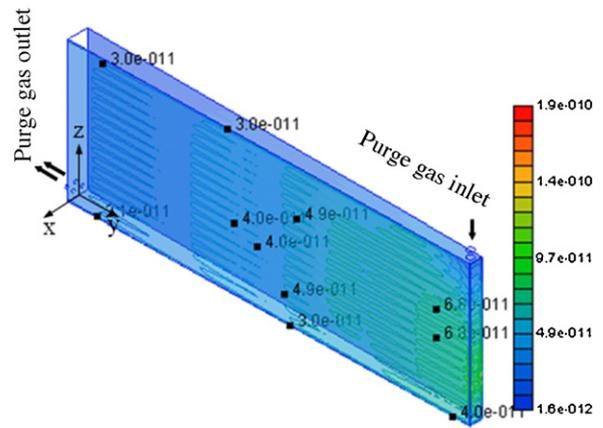
Fig. 9. The tritium permeation flux at the purge gas–structure interface.
