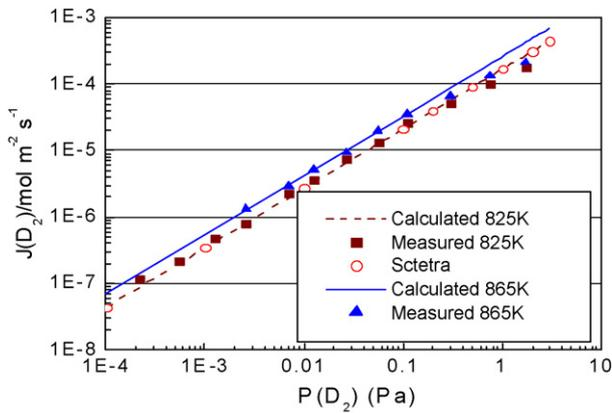
Fig. 2. D<sub>2</sub> permeation flux as a function of the upstream deuterium pressure.
