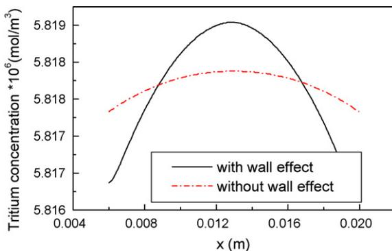
Fig. 8. The tritium concentration with and without wall effects along the x-direction at y=0.2 m and z=0.0672 m.
