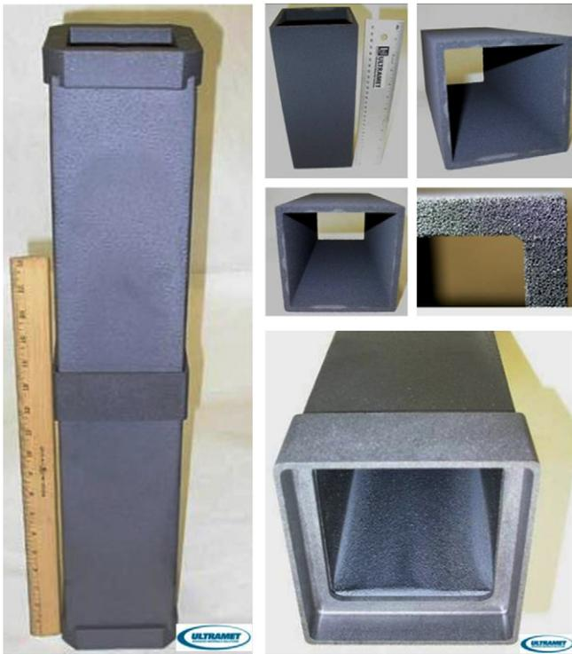
**Fig. 4.** FCI prototype consisting of an assembly of two FCI segments totaling a height of 635 mm, 116 mm wide, and 116 mm deep; the SiC-foam was infiltrated by CVI SiC to ~10–20 vol% (Ultramet, Inc.).
