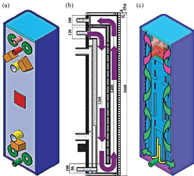
**Fig. 1.** (a) DCLL TBM module. (b) Poloidal Pb-17Li flow, inlet and outlet channels located at the top (c) Helium flow distribution at the back to the first wall, inlet located at the bottom and outlet located at the top of the module.
