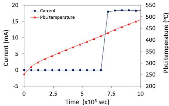
Fig. 3. Electrical insulation test result (Run #2).
