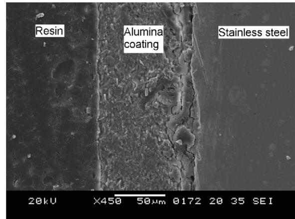
Fig. 5. SEM image of the  $\text{Al}_2\text{O}_3$  coating cross-section without experience of molten PbLi exposure during the electrical insulating test.
