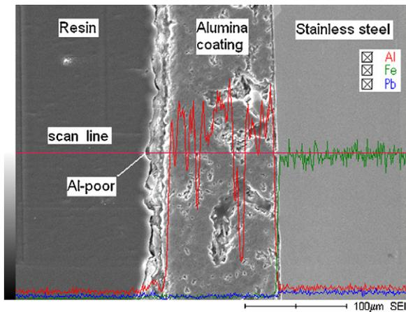
**Fig. 6.** SEM image of the  $\text{Al}_2\text{O}_3$  coating cross-section with experience of molten PbLi exposure during the electrical insulating test.
