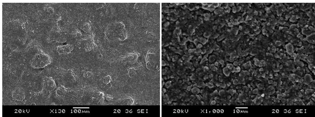
Fig. 4. SEM images of the  $\text{Al}_2\text{O}_3$  coating surface (left:  $\times 130$ , right:  $\times 1000$ ).
