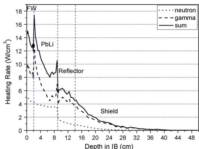
Fig. 5. Nuclear heating for Case 1.
