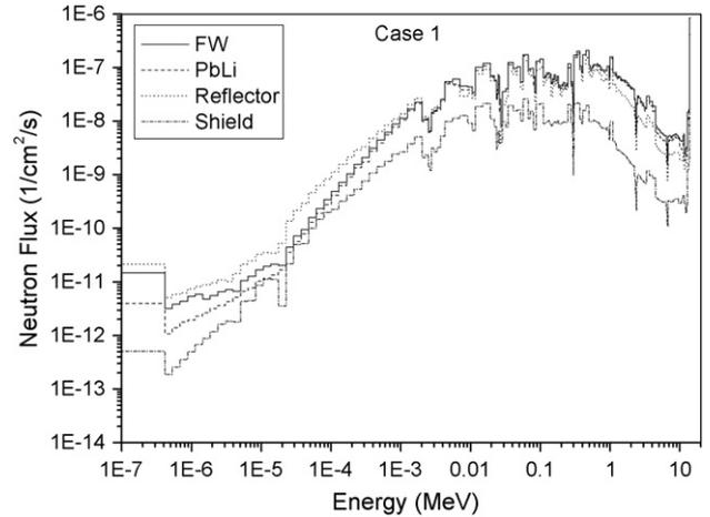
Fig. 2. Region averaged neutron flux for Case 1.
