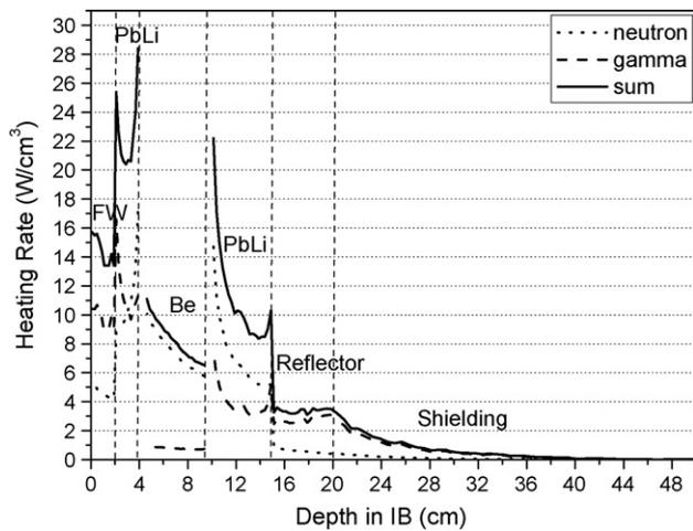
Fig. 6. Nuclear heating for Case 5.
