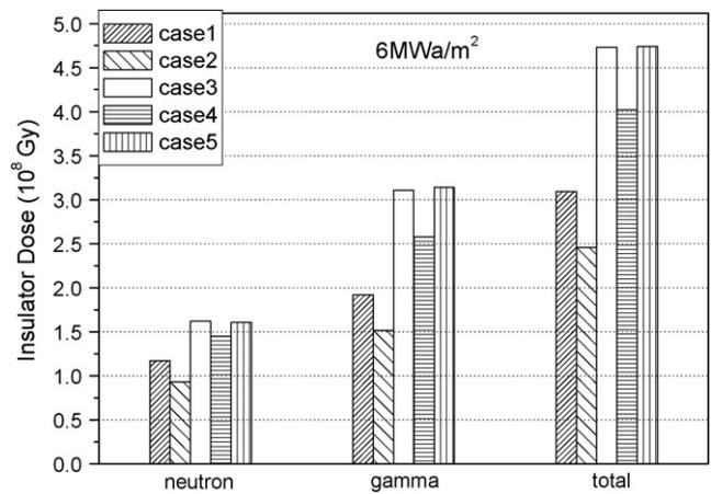
Fig. 4. Peak dose with spinel insulator.
