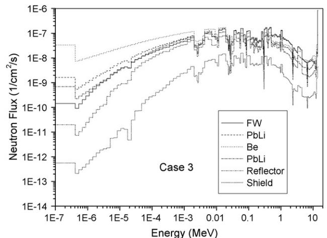
Fig. 3. Region averaged neutron flux for Case 3.
