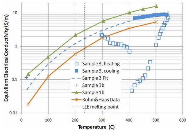
Fig. 6. Equivalent electrical conductivity of Sample 3 assuming  $r_c = 0$  in Eq. (1).
