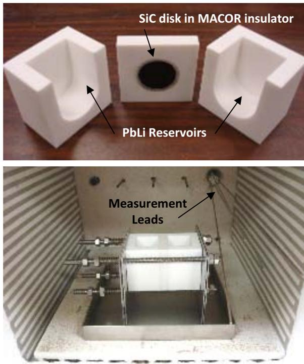
Fig. 1. LLE/SiC DC resistance measurement apparatus in pieces (above) and partially assembled furnace (below).
