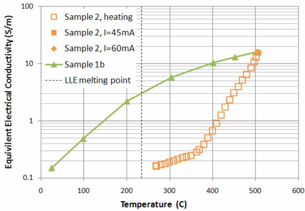
Fig. 5. Equivalent electrical conductivity of Sample 2 assuming  $r_c = 0$  in Eq. (1).
