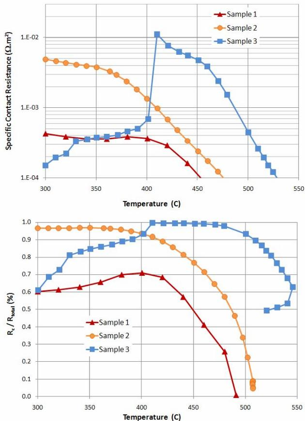
Fig. 7. Specific contact resistance of test samples using estimates of intrinsic electrical conductivity measured on Sample 1b: absolute  $r_c$  (above) and percentage of total sample resistance due to contact resistance (below).
