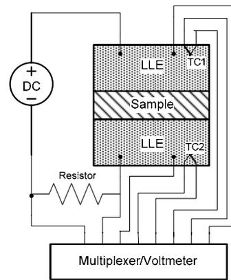
Fig. 2. DC resistance test circuit with LLE electrodes
