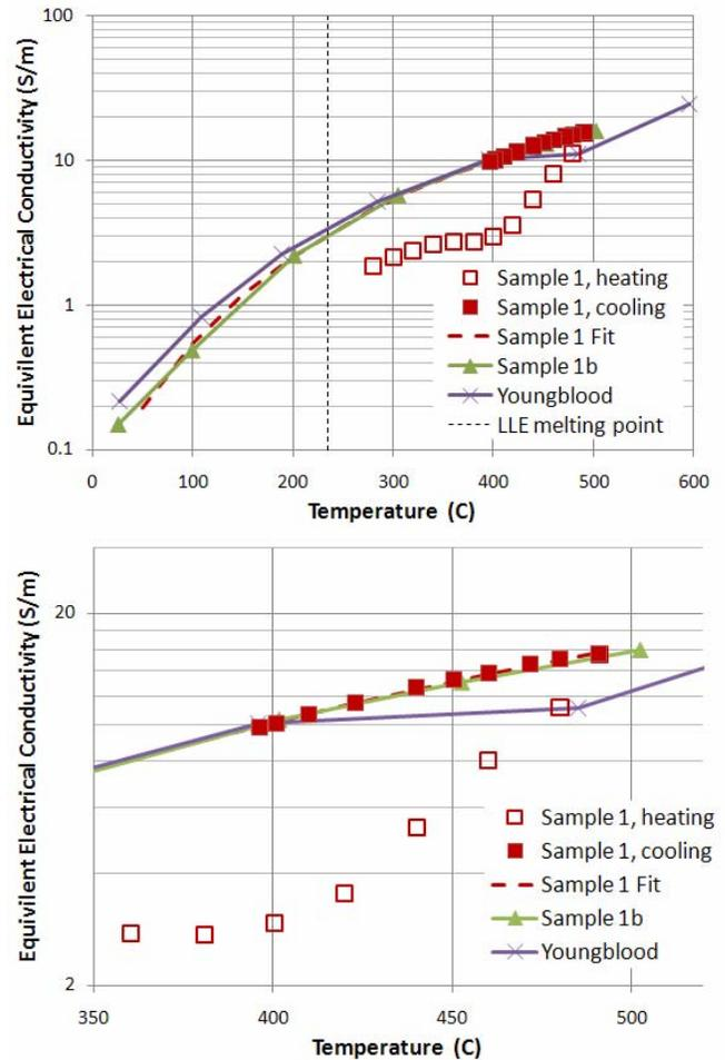
Fig. 4. Equivalent electrical conductivity of Sample 2 assuming  $r_c = 0$  in Eq. (1). The data were measured during the initial heat up to ~500C (open symbols), and then upon cooling (closed symbols). For comparison, Youngblood and bar Sample 1b are also shown: Full temperature range (above), reduced range (below).
