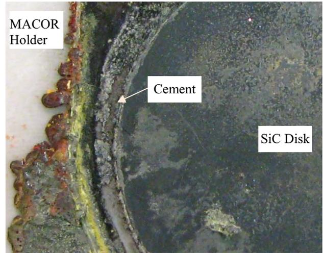
Fig. 8. Image of portion of SiC disk and MACOR sample holder showing greenish scale on SiC and colorful compounds formed by LLE attack on the MACOR.
