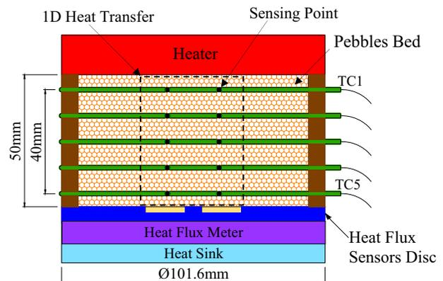
Fig. 1. The pebble bed and its thermocouples.
