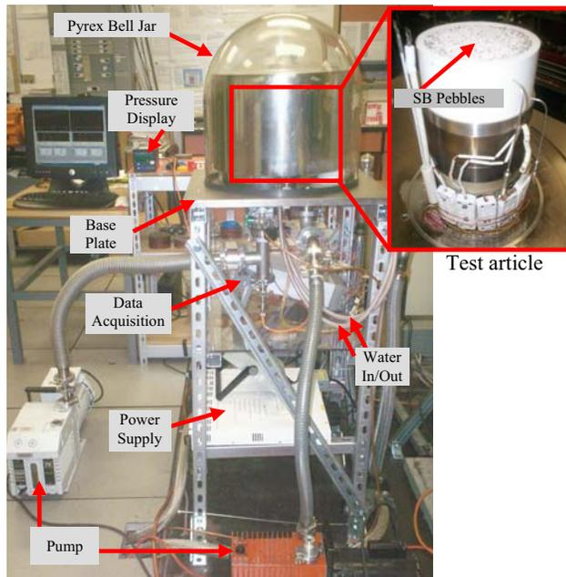
Fig. 2. The experimental apparatus.
