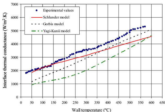
Fig. 3. Interface conductance of the  $\text{Li}_2\text{TiO}_3$  pebble bed.
