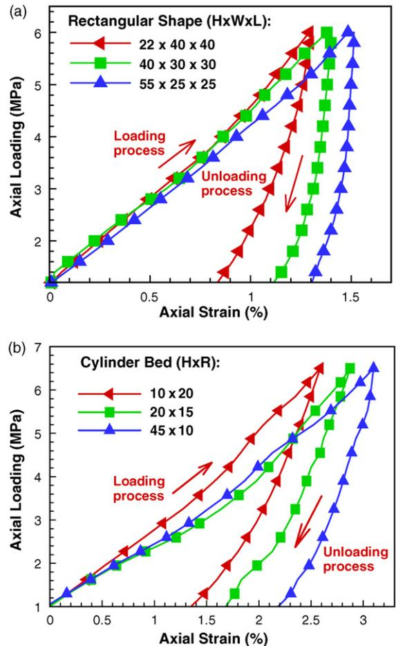
Fig. 3. Effect of bed geometry on the mechanical behaviors of the pebble beds. (a) rectangular pebble beds; (b) cylinder pebble beds.
