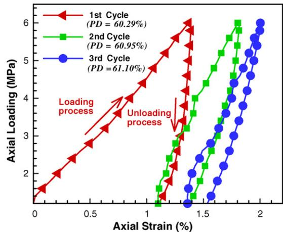
Fig. 2. Packing density effects on mechanical behaviors of the pebble beds.
