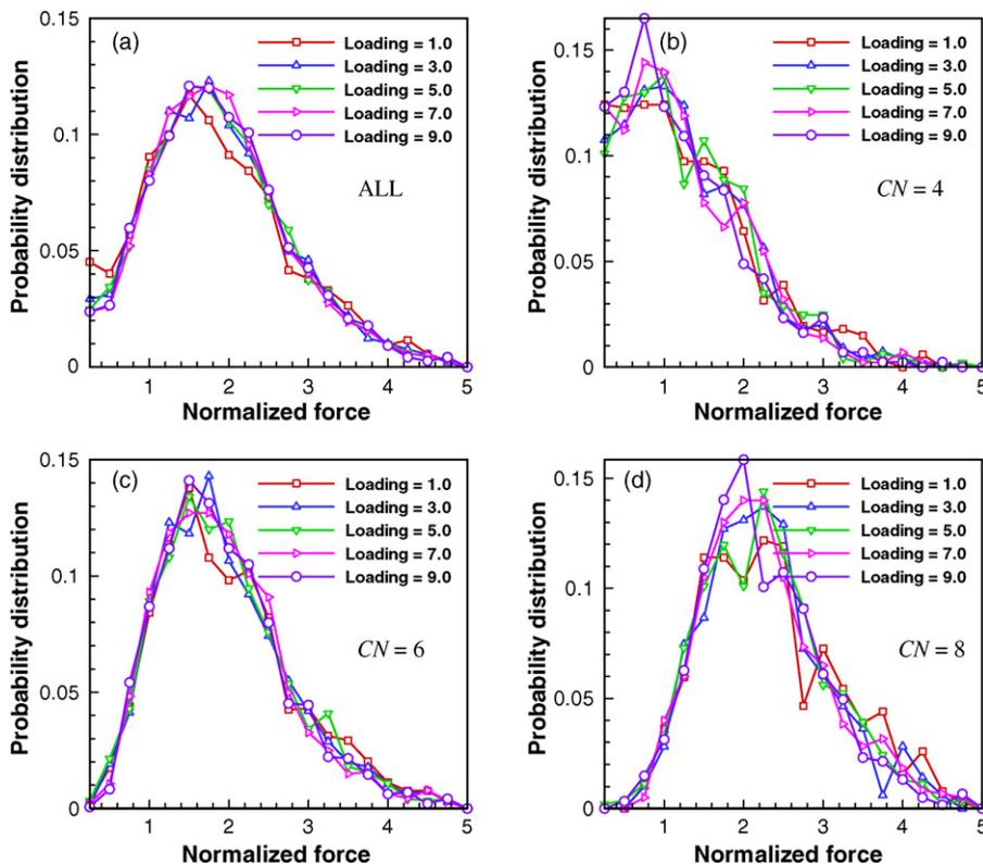
Fig. 4. Probability distribution of the maximal contact forces under different compaction loading (loading unit: MPa). (a) All together; (b) CN=4; (c) CN=6; (d) CN=8.
