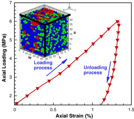
Fig. 1. Stress–strain behaviors of granular materials in a rectangular box under uniaxial compaction (initial packing density 60.3%; total particle number 5000;  $H \times L \times W$  is  $35 \times 30 \times 30$ ).
