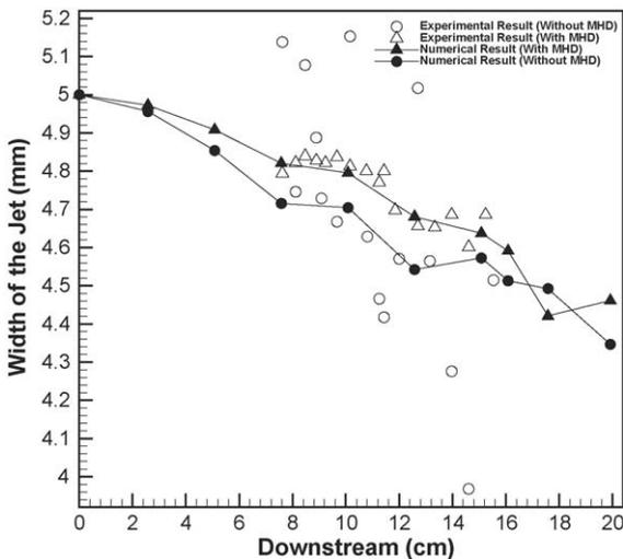
Fig. 2. Radius of the jet with/without magnetic field downstream (initial velocity: 3 m/s).
