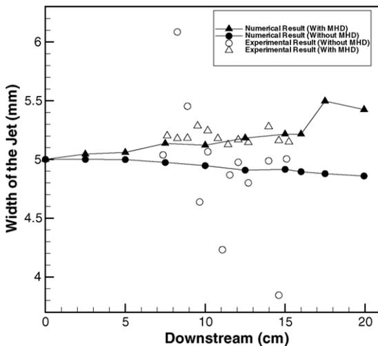
Fig. 6. Radius of the jet with/without magnetic field downstream (initial velocity: 5 m/s).
