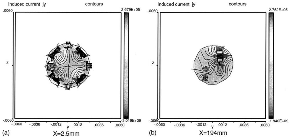
Fig. 3. Contours of induced current in X-direction (initial velocity: 3 m/s).
