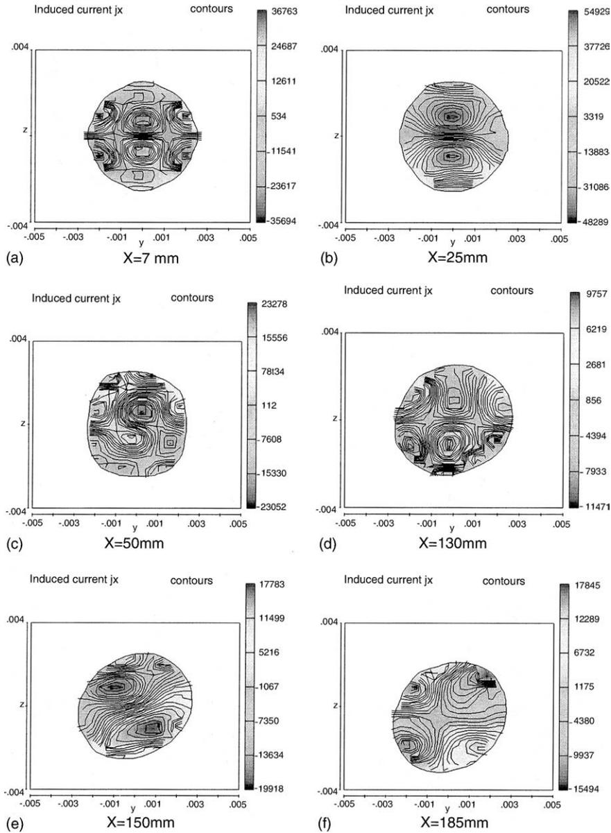
Fig. 7. Contours of induced current in X-direction downstream (initial velocity: 5 m/s).
