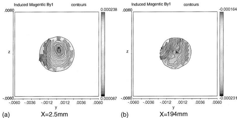
Fig. 4. Contours of induced magnetic field in X-direction (initial velocity: 3 m/s).
