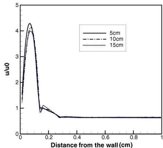
Fig. 2. Velocity variation with distance from the wall.
