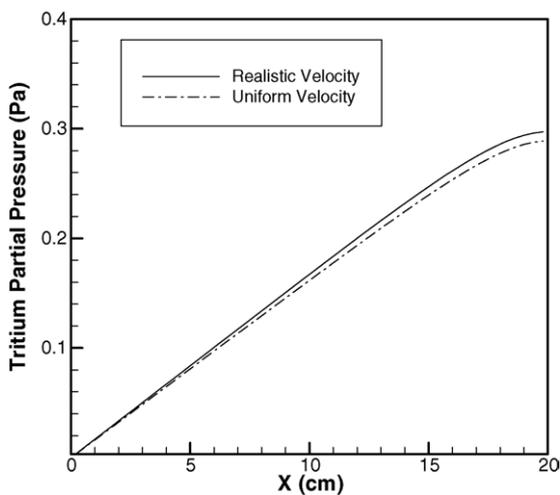
Fig. 5. Averaged tritium partial pressure along the flow direction (3D results).
