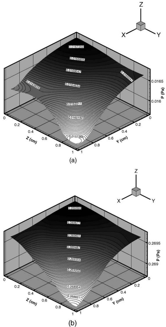
Fig. 6. Tritium partial pressure profile at different flow locations: (a) near the inlet (tritium partial pressure ~ 0.0165 Pa); (b) near the outlet (tritium partial pressure ~ 0.269 Pa).
