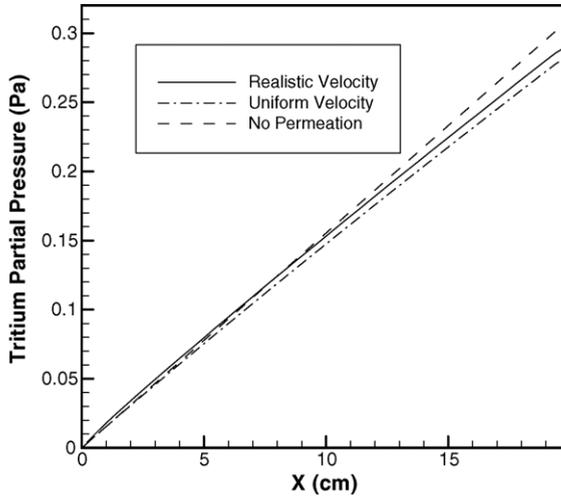
Fig. 7. Average tritium partial pressure along flow direction with lower diffusivity.
