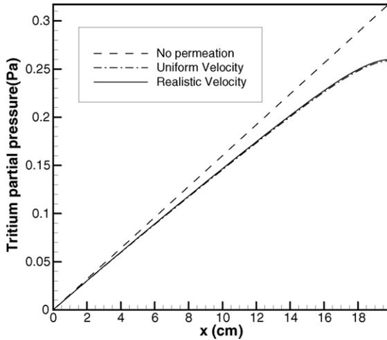
Fig. 3. Average tritium partial pressure along purge gas flow direction.
