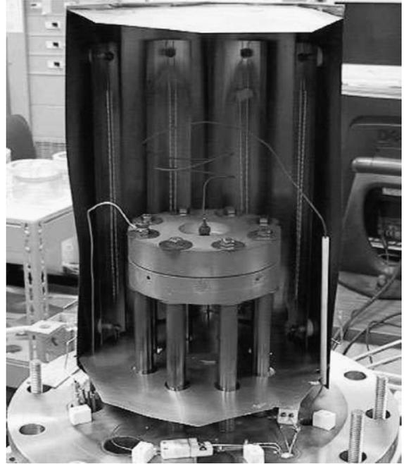
Fig. 1. Test article inside high temperature furnace.
