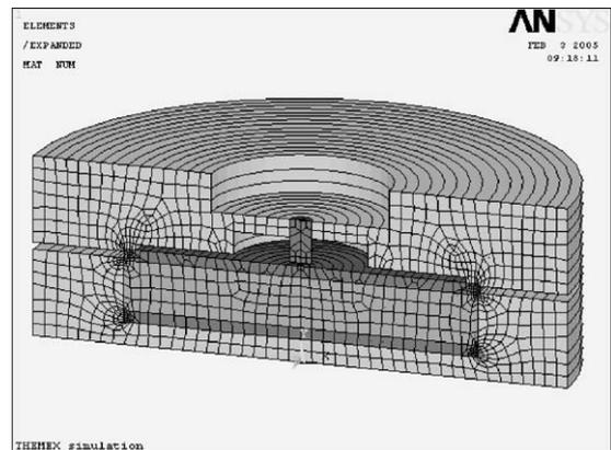
Fig. 2. Test article schematic and finite element meshing.
