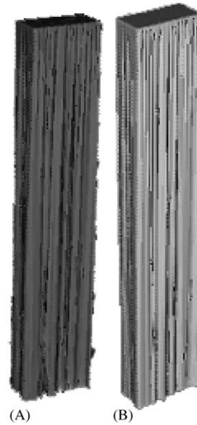
Fig. 2. Simulation of typical IFE grid jets with We and Re \sim 10^5 with inlet conditions: (A) flat, average-velocity profile and (B) “turbulent-like” flatter average-velocity profile.
