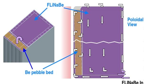
Fig. 1. Schematics of the self-cooled  $\text{FLiNaBe}$  design.
