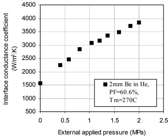
Figure 8. Effect of external applied pressure on Be-SiC interface conductance coefficient
