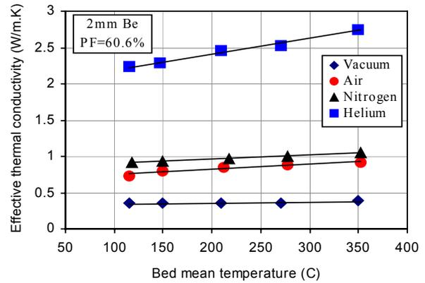
Figure 5. Effective thermal conductivity of beryllium bed with different cover gases
