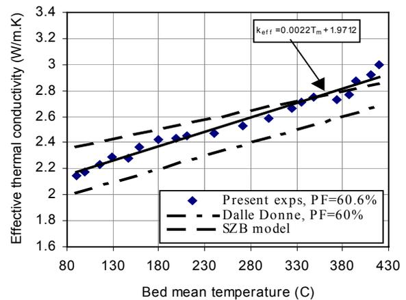
Figure 3. Bed effective thermal conductivity as a function of the bed mean temperature
