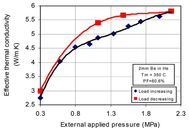
Figure 7. Bed effective thermal conductivity with load increasing and decreasing
