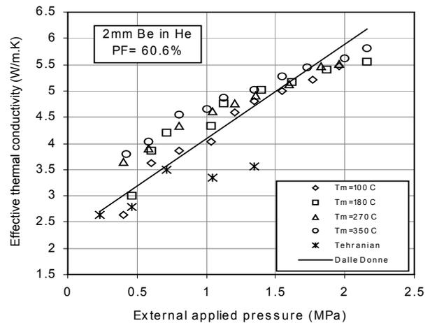
Figure 6. Effect of external applied pressure on beryllium bed effective thermal conductivity
