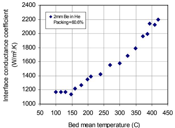
Figure 4. Interface conductance coefficient as a function of the bed mean temperature
