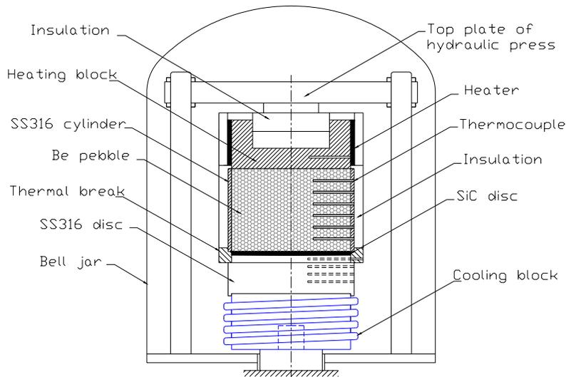
Figure 1. Schematic drawing of the experimental apparatus
