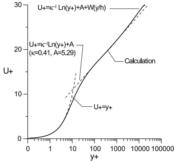
Fig. 6. Test 1. Calculated against theoretical velocity profile [29] in open channel flow without a magnetic field:  $Re = 500000$ .
