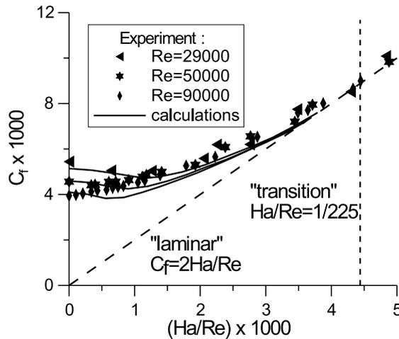
Fig. 2. Experimental [21] and calculated friction factor results for a wall-normal magnetic field.
