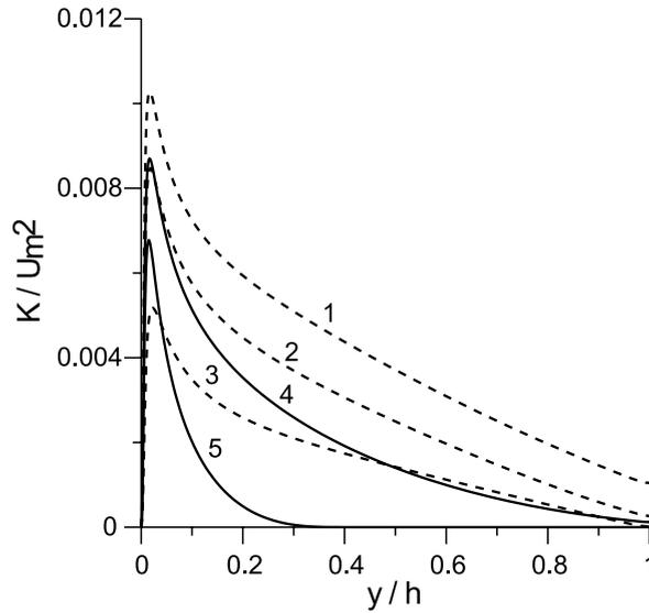
Fig. 9. Distributions of the turbulence kinetic energy in a chute MHD flow:  $Re = 30000$ . 1 –  $Ha = 0$ ; 2 –  $Ha = 30$ , spanwise magnetic field; 3 –  $Ha = 50$ , spanwise magnetic field; 4 –  $Ha = 20$ , wall-normal magnetic field; 5 –  $Ha = 40$ , wall-normal magnetic field.
