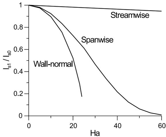
Fig. 4. Decrease of the dissipation length scale at the free surface under the influence of a magnetic field:  $Re = 30000$ .
