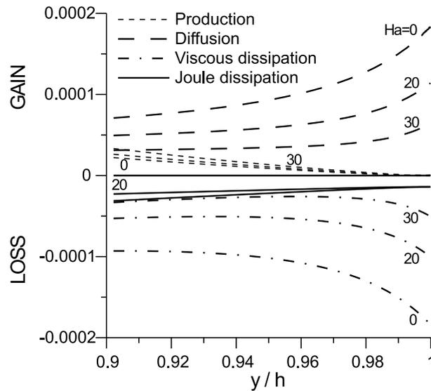
Fig. 8. Budget of the turbulence kinetic energy in the free surface region of a chute MHD flow in a spanwise magnetic field:  $Re = 30000$ .
