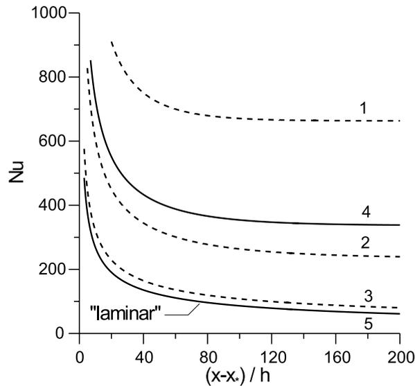
Fig. 12. Nusselt number in a chute MHD flow with the heat flux applied to the free surface:  $Re = 30000$ ;  $Pr = 30$ . See notation in Fig. 9.
