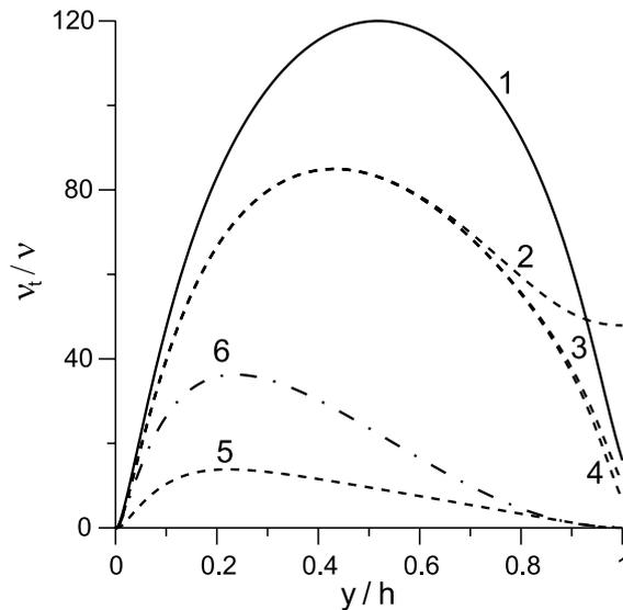
Fig. 5. Distributions of the eddy viscosity in open channel MHD flow calculated with different free surface boundary conditions: 1 –  $Ha = 0$ , Hossain and Rodi BC (11); 2 –  $Ha = 25$ , spanwise magnetic field, symmetry BC (10); 3 –  $Ha = 25$ , spanwise magnetic field, Hossain and Rodi BC (11); 4 –  $Ha = 25$ , spanwise magnetic field, modified Hossain and Rodi BC (13); 5 –  $Ha = 60$ , spanwise magnetic field, symmetry BC (10); 6 –  $Ha = 25$ , wall-normal magnetic field, symmetry BC (10).
