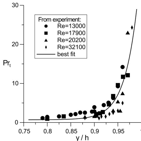
Fig. 11. Distribution of the turbulent Prandtl number in the free surface region of open channel flow based on the experimental data for the eddy diffusivity for heat [31] and present calculations of the eddy diffusivity for momentum.
