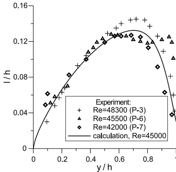
Fig. 7. Test 2. Calculated against experimental [30] dissipation length scale in open channel flow without a magnetic field.
