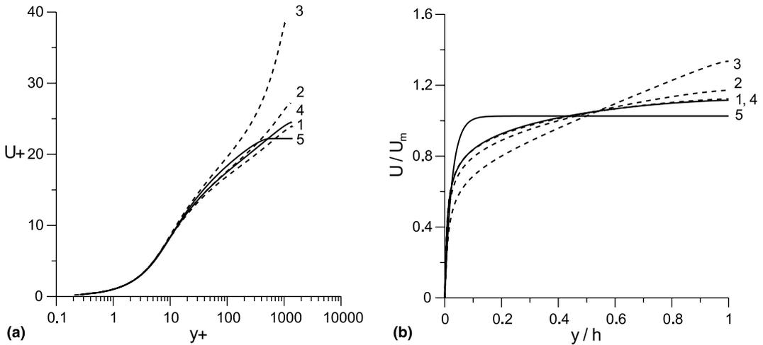
Fig. 10. Velocity profiles in a chute MHD flow plotted with universal (a) and outer (b) scaling:  $Re = 30000$ . See notation in Fig. 9.
