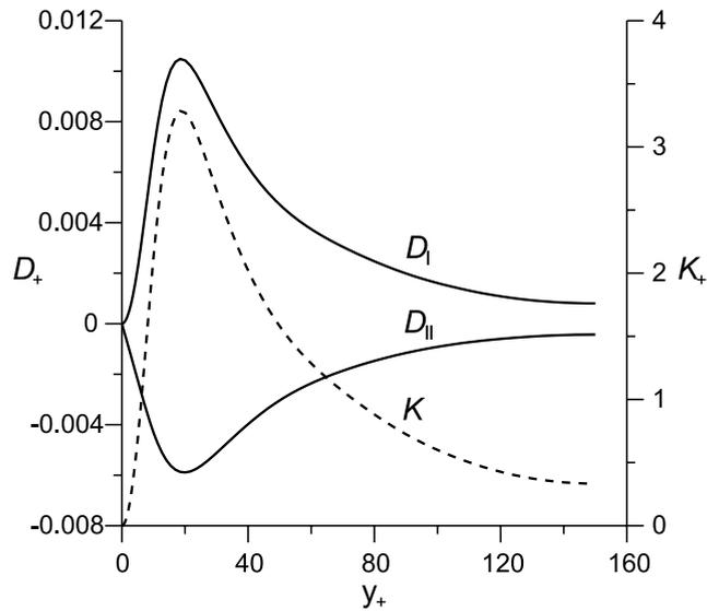
Fig. 1. Distributions of the  $D_{\perp}$  and  $D_{\parallel}$  terms entering the expression (3) for the Joule dissipation and the turbulence kinetic energy distribution in fully developed MHD flow between parallel walls with a wall-normal magnetic field [10]:  $Ha = 6$ ;  $Re_{\tau} = 150$ .
