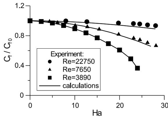
Fig. 3. Experimental [22] and calculated friction factor results for a spanwise magnetic field.
