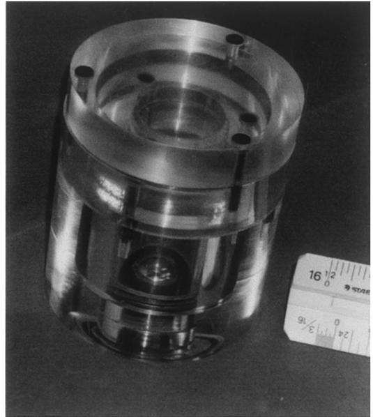
Fig. 2. Target assembly for a liquid-fracture strength experiment called ‘Popoff’ at UCLA. This experiment measures the fracture strength of characteristic liquids such as Li, Pb, Flibe, and LiPb. Loaded by rapid tensile strains typical of shock loaded and rapidly heated thick jets and thin films in IFE wall protection schemes.
