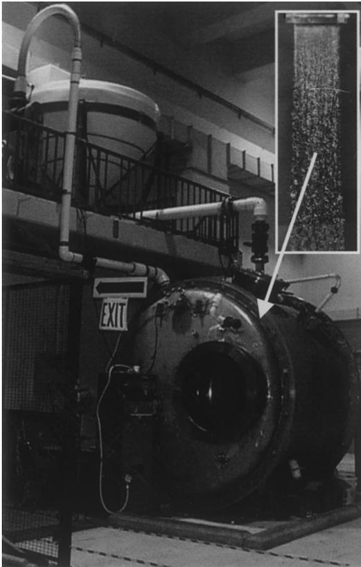
Fig. 1. This UCB facility uses transient flow into a large vacuum vessel to study single jets (currently) and partial-liquid pockets with a few jets (future plans). Water can be used to simulate Flibe jets at  $1/2$ – $1/4$  geometric scale with dimensionless  $Re$ ,  $Fr$  and  $We$  numbers matching those in a power plant chamber.
