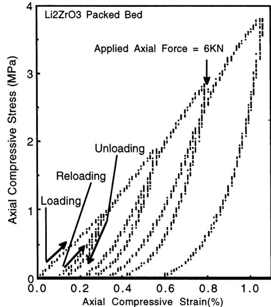
Fig. 2. Stress vs. strain during cyclic loading and unloading tests (initial bed packing density = 57.5%).
