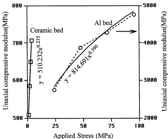
Fig. 4. Compressive modulus as a function of applied stress.
