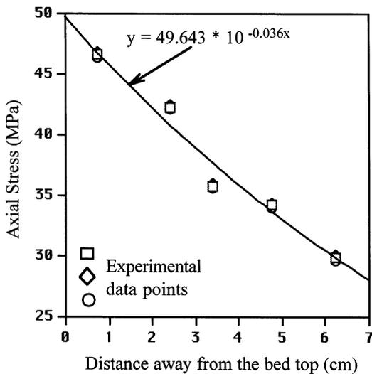
Fig. 6. Axial local stress as a function of distance away from the bed top (aluminum packed bed).
