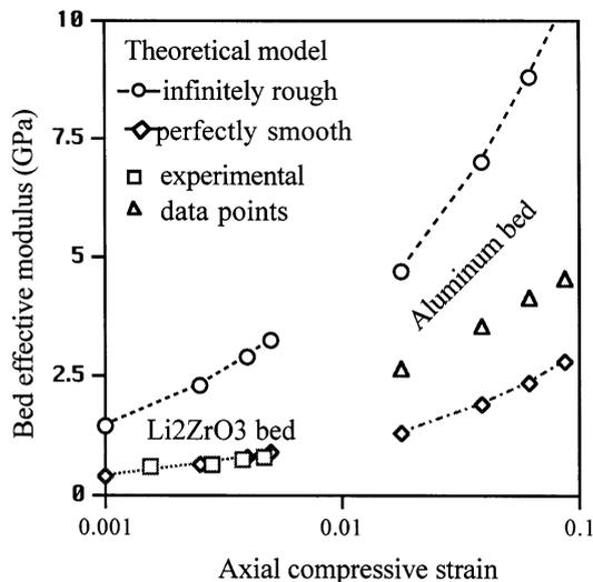
Fig. 7. Comparison of experimental data of effective modulus with theoretical curves.
