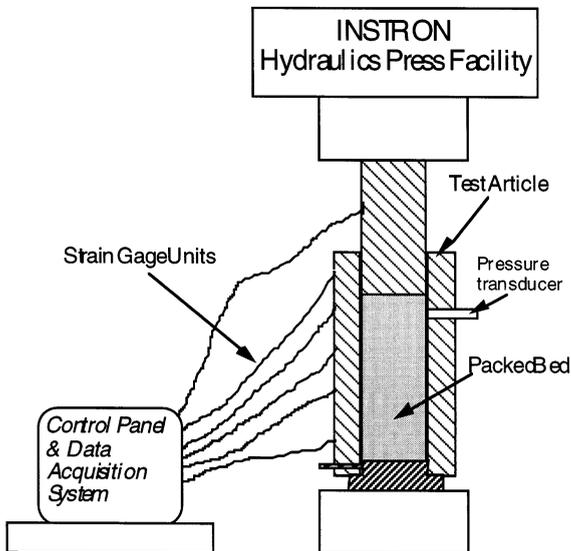
Fig. 1. Uniaxial compression test facility.
