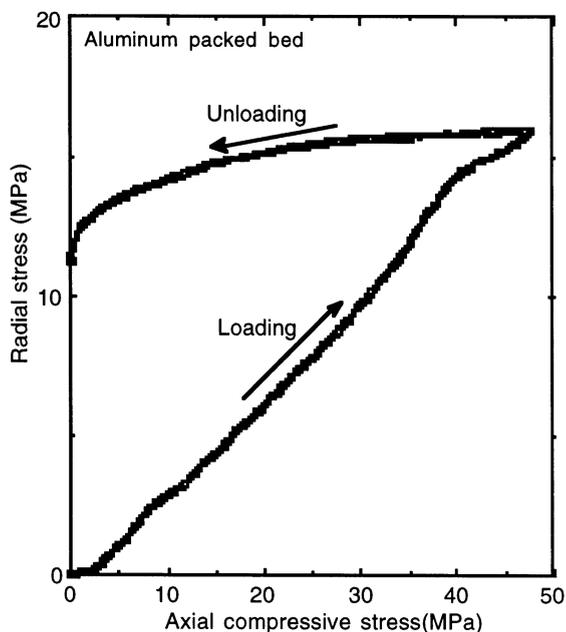
Fig. 5. Radial local stress vs. axial local stress (at top of the bed) during loading and unloading of aluminum packed bed.
