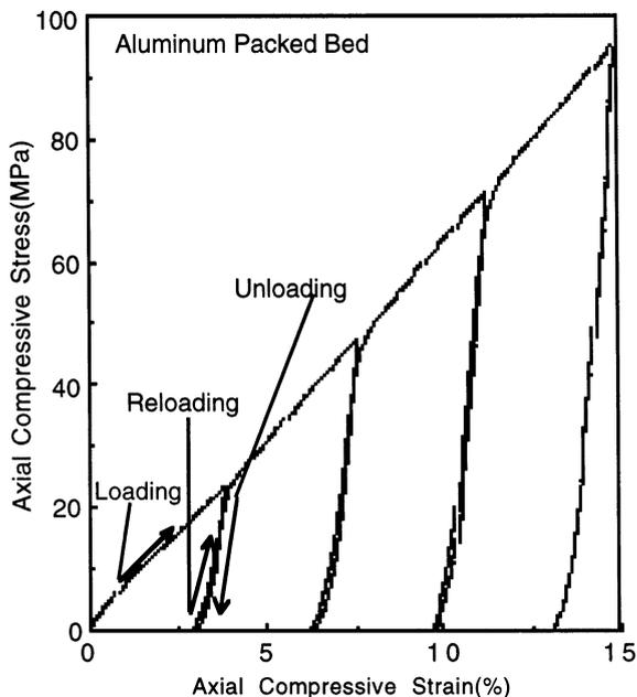
Fig. 3. Stress vs. strain during cyclic loading and unloading tests (initial bed packing density = 59.0%).
