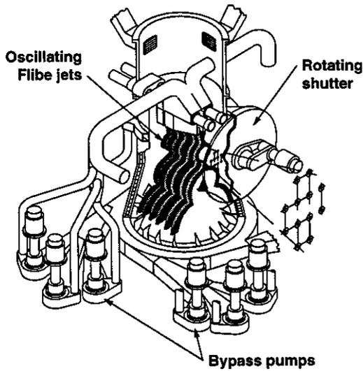
Fig. 5. The HYLIFE-II chamber uses an array of oscillating jets of liquid Flibe to form a thick protective blanket between the fusion target and the chamber structures. The pumps required to circulate the Flibe ( $\text{Li}_2\text{BeF}_4$ ) are shown.
