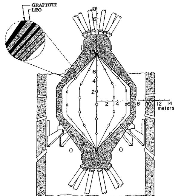
Fig. 1. The Sombrero chamber features carbon–carbon composite first wall and blanket structures. Flowing Li<sub>2</sub>O is the breeder and coolant.
