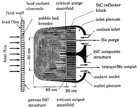
Fig. 3. Prometheus chamber features a Pb-cooled porous SiC first wall and a helium-cooled  $\text{Li}_2\text{O}$  breeding blanket with SiC structures.
