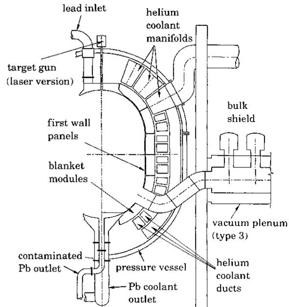
Fig. 4. A steel vacuum vessel contains the Prometheus FW and blanket modules. Inlets and outlets for the lead and helium coolants are shown as well as the vacuum port for pumping non-condensable gases.
