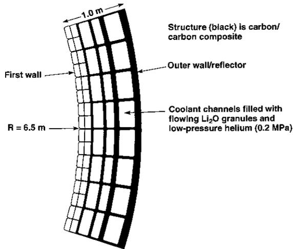
Fig. 2. Cross-section of the Sombrero blanket showing the channels for the flowing  $\text{Li}_2\text{O}$  breeder-coolant (open regions) and the carbon-carbon composite structure (dark regions).
