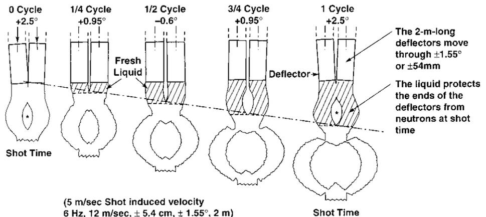
Fig. 6. Sequence showing how the liquid pocket is formed using the oscillating nozzles.
