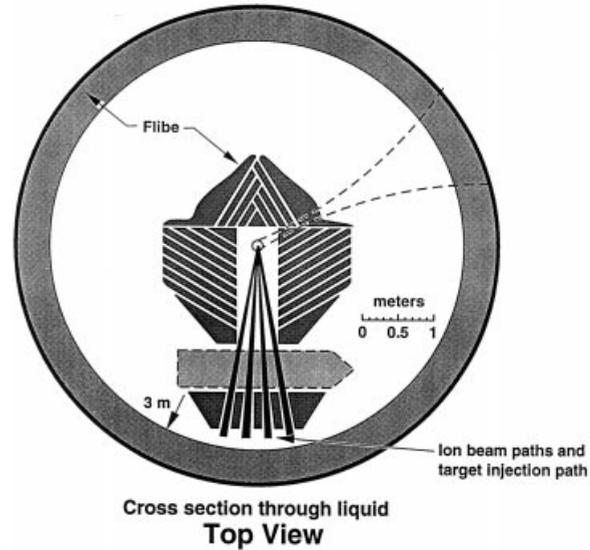
Fig. 7. Cross section of the chamber at the target elevation showing the open space for vapor venting and 0.5 m of liquid to attenuate neutrons in all directions except the beam paths. (The single-sided illumination configuration is shown, although two-sided illumination is now the preferred approach).
