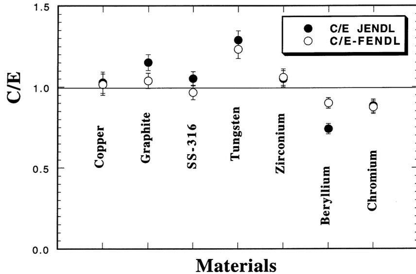
Fig. 6. C/E values for the total nuclear heating of other probe materials at the first location in the copper assembly.
