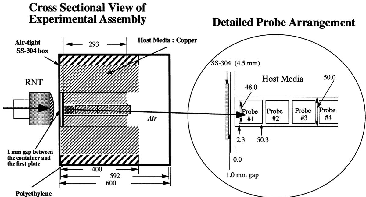
Fig. 1. The copper experimental assembly for the nuclear heating measurement by the calorimetric technique. Dimensions given in the figure are in millimeters.
