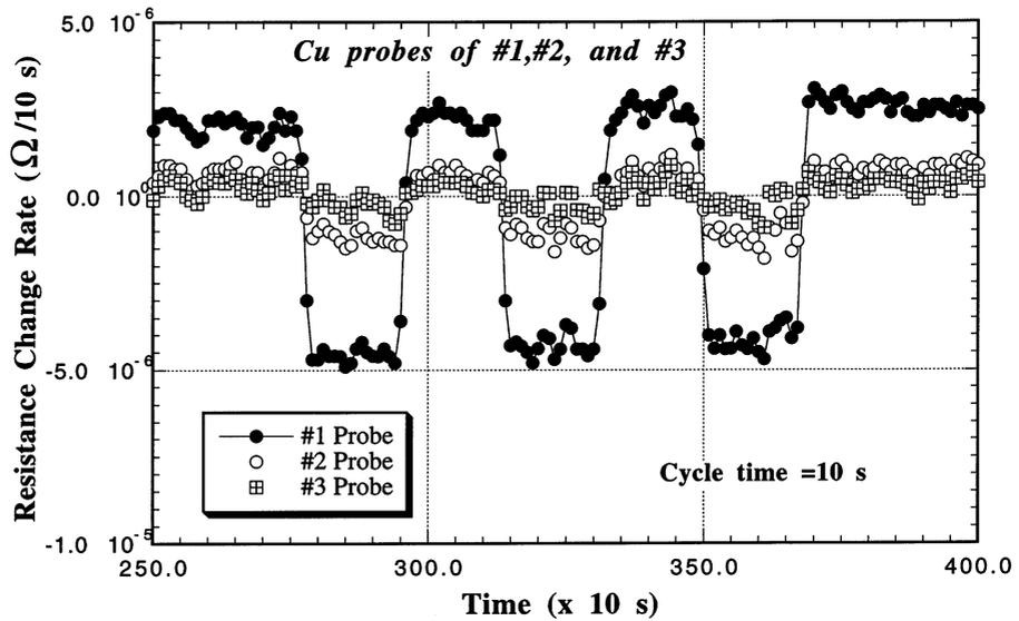
Fig. 2. Derivatives of the temperature rise data on the first copper probes. The rectangular shape drops in the derivatives correspond to the temperature rise due to nuclear heating by D-T neutron irradiations.
