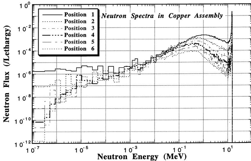
Fig. 3. Neutron spectra at various depths in the copper assembly calculated by MCNP with the FSXLIB-J32 JENDL-3.2 based nuclear library.
