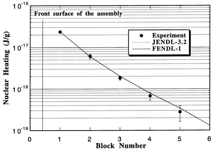
Fig. 4. Measured total nuclear heating distribution along the central axis of the copper assembly. The results of calculations by JENDL and FENDL are shown for comparison.
