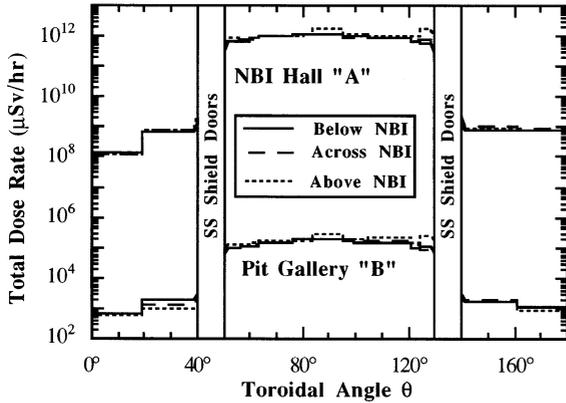
Fig. 4. Toroidal variation of the total operational dose rate for regions below, across, and above the NBI ports within the NBI Hall, A, and Pit Gallery, B.
