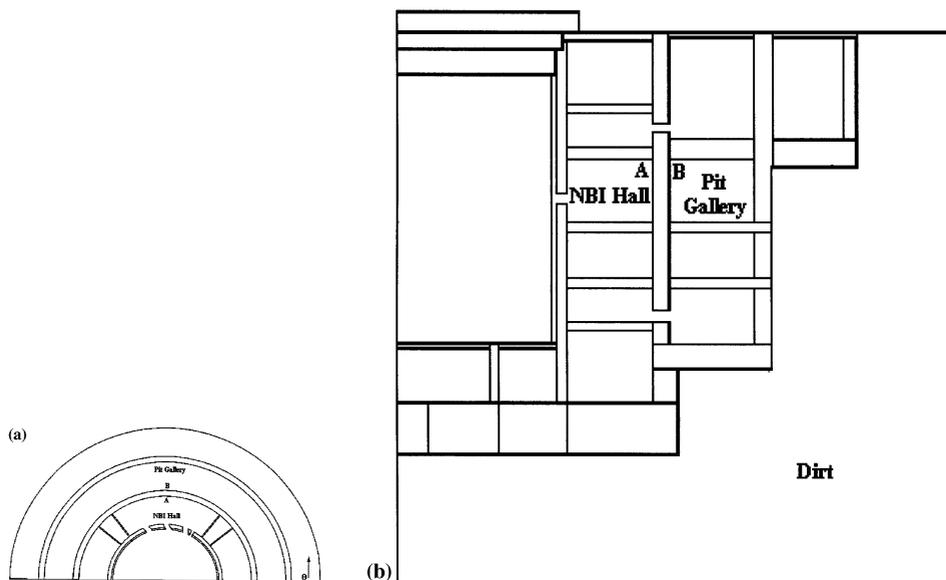
Fig. 2. (a) X-Y view of the MCNP building model at the equatorial level ( $Z = -20$  m). (b) Y-Z view of the MCNP building model. Note, A and B in the NBI Hall and Pit Gallery are the locations of the tally surfaces.
