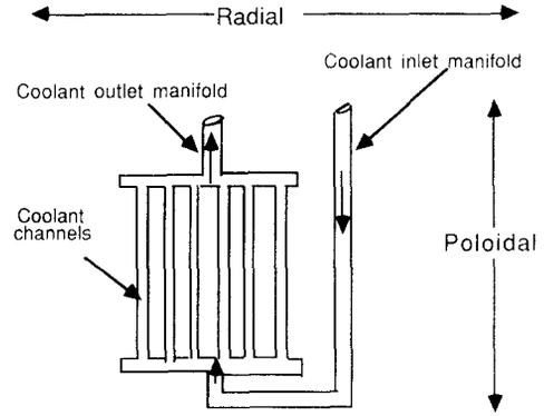
Fig. 2. An example of a poloidally oriented channel arrangement inside a blanket segment.
