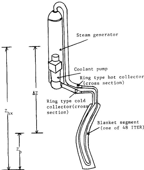
Fig. 1. Illustration of a poloidally oriented outboard blanket primary cooling system (one of the loop).
