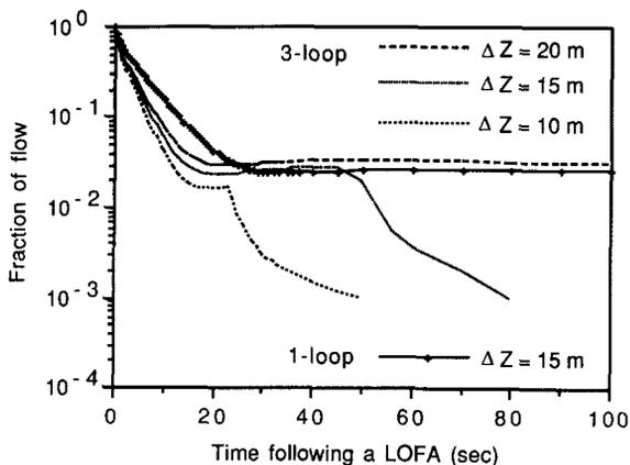
Fig. 3. Transient flow behaviors following a LOFA for different hydrostatic heads (ITER layered pebble bed design concept).
