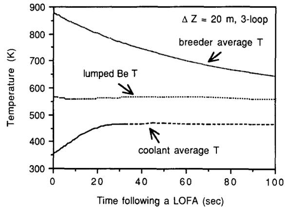
Fig. 4. Temperature histories of solid breeder, lumped Be region and of coolant following a LOFA for hydrostatic head of 20 m, 3-loop system.
