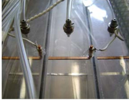
Figure 2: copper electrodes used to measure flow rates in each channel
